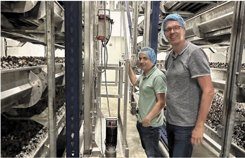
Figure 2. Picking lorries attached to the shelves are hooked up to a tensioned harvest belt which runs the length of the room, demonstrated here by Tom Peeters and Dennis Tros from GTL Europe. Note that the picking lorries are also used to irrigate the beds.
