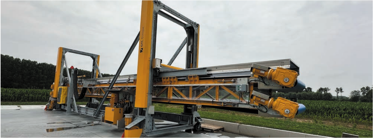
Figure 5. The transfer bridge used to move half a bed at a time from the pinning rooms to harvest rooms, the harvest rooms being equipped with tilting shelves.
