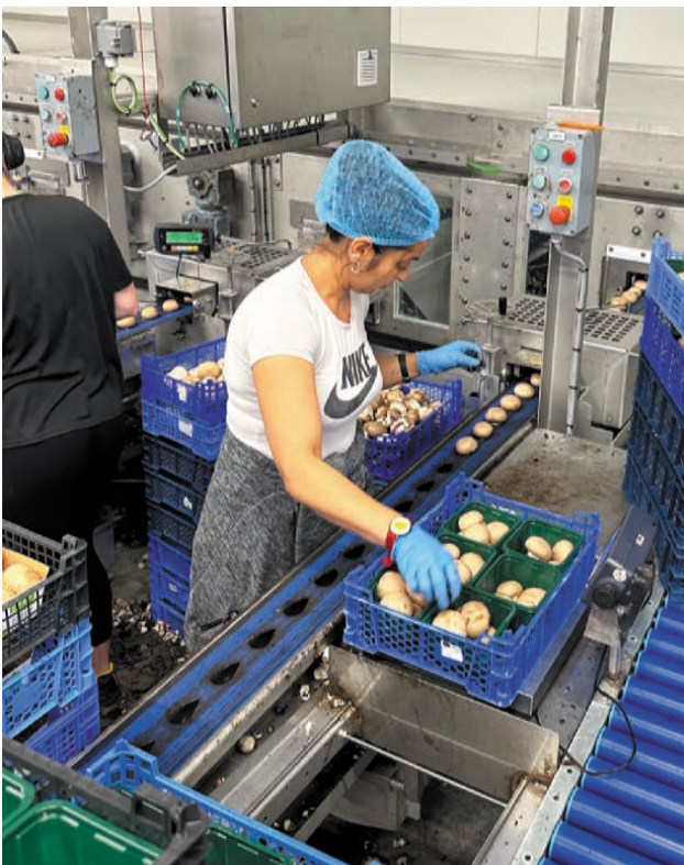
Figure 4. Mushrooms are trimmed as they pass into the packing area, where a packer transfers mushrooms from the belts into punnets.
