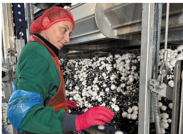
Figure 6. the tilting shelves allow pickers to stand upright and use both hands, reducing strain and improving picking rates.
