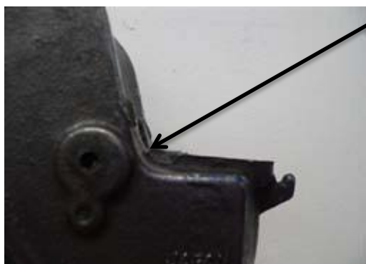
Photo 3 (below): Steering bracket with the turning stop removed
