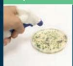
Disinfect the disc with BKC80, 20% solution after first reading to ensure biosafety.
