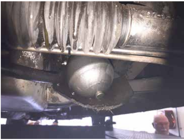
Now for the brake spheres. The second one is hidden right behind
