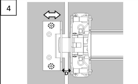
4 Adjust the position of the frame until a distance of D= 19/32" (in case of use T391 or T393 panic device D=43/64") from the panic device mechanism, verify that both are parallel and adjust the screws.
