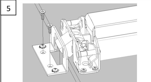
5 Mark and drill as mentioned in the template for the placement of the flat head fixing screws (Parker n°7x5/8"). Fix them tightly.
