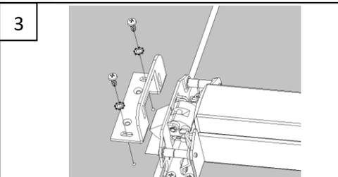
3 Install the panic device according it's to instruction manual. Fit the center case with its screws (Parker # 8x1/2") and washers according to the sequence shown in the image.
