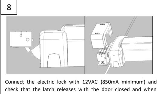
8 Connect the electric lock with 12VAC (850mA minimum) and check that the latch releases with the door closed and when opened allows free passage. Finally put on the pressure cap.
