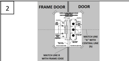
2 Present the template according to the corresponding panic device, drill the holes and fretwork. Use scotch tape to fix the template.
