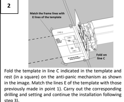
2 Fold the template in line C indicated in the template and rest (in a square) on the anti-panic mechanism as shown in the image. Match the lines E of the template with those previously made in point 1). Carry out the corresponding drilling and setting and continue the installation following step 3).
