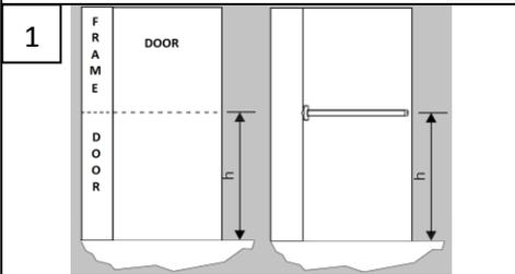
1 To mark mechanism height (h), place bar at a height between 36" (900mm) and 43" (1100mm) from the floor. In case of use a three point latches panic device and the door height is more height that 7', use h=43".
