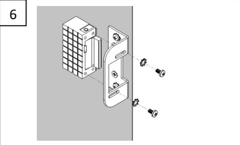
6 Fit the electric lock with its screws (M4x8) and washers according to the sequence shown in the image
