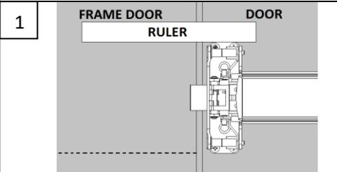
1 Remove cap case from the corresponding panic device installed. Drawing a line parallel to the upper and lower edges of the panic device mechanism, the use of a ruler is recommended.
