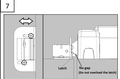
7 With the door closed, adjust the position of the electric latch so that there is no gap between the panic device latch and electric lock latch. The electric lock latch must be not loaded when the door it close, because the electric lock not open in this way. Use a door closer.
