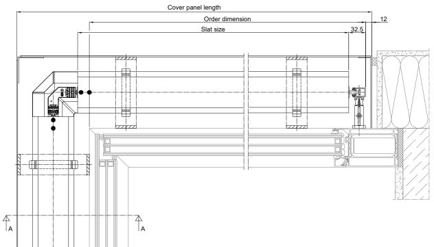
The greyed-out sections of the illustration represent interfaces to general trades which, on the whole, must be planned and performed independently and on-site. WAREMA does not provide services for the greyed-out interfaces and assumes no liability for them.
