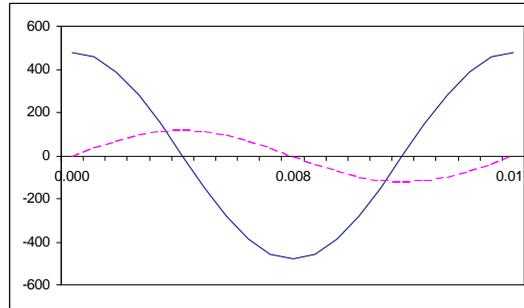
**Figure 2. Effect of power factor upon voltage (—) and current (---) waveforms.**
