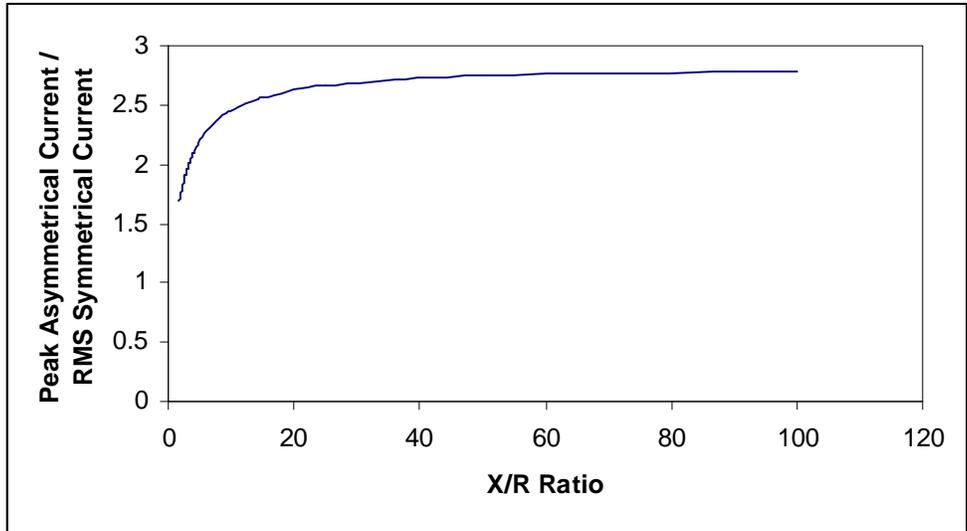
**Figure 4. Peak asymmetrical current as a function of symmetrical RMS current. (Data taken from notes on the GE Electrical Distribution & Control Low-voltage Protector Application Seminar.)**
