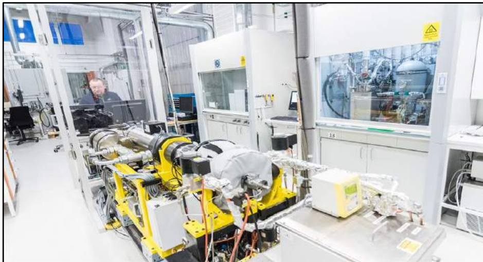
Fig 4. Ammonia Engine being testing at Wärtsilä R&D [12]
