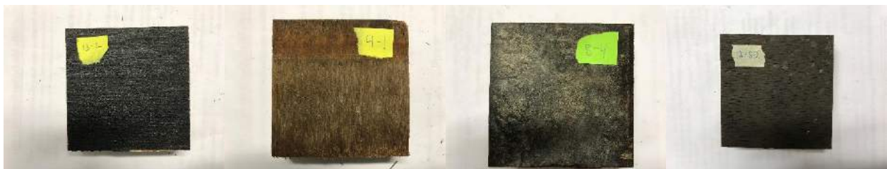
Figure 2: Examples of the plywood samples made for the Cone Calorimeter tests.
