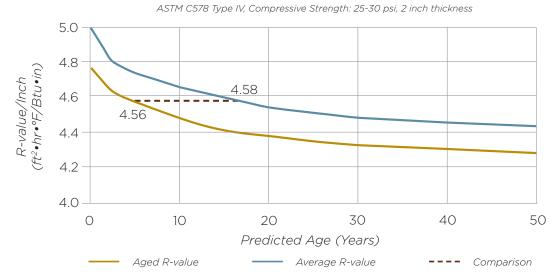
Applying ASTM C1303, a sample of XPS insulation obtained commercially was evaluated and the predicted aged R-value determined. A comparison was made between the 5-year (point-in-time) aged R-value and the 15-year average R-value to demonstrate their equivalence as noted in ASTM C1303, Section 5.4. The 5-year aged R-value of 4.56 agreed quite well with the 15-year average R-value of 4.58 (see chart above).
