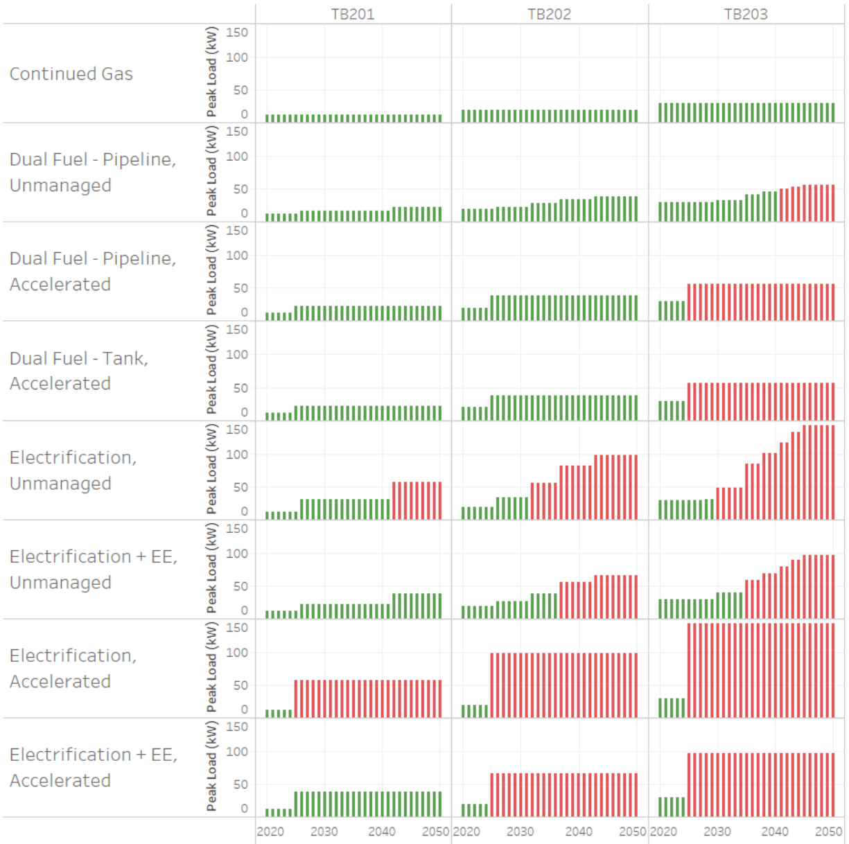
Figure 9. Peak loads for the multifamily segment's three transformers under each scenario. Green represents peak load below the rated transformer capacity; red signifies the transformer capacity is exceeded.
