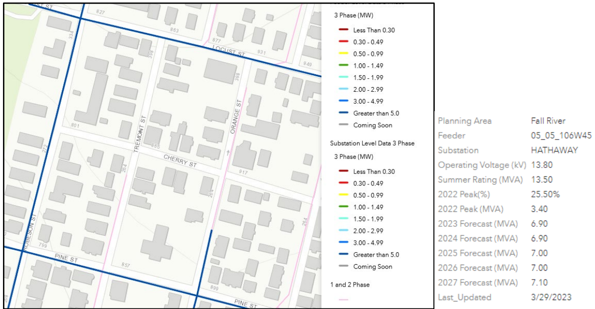
Figure 10. National Grid Hosting Capacity Map (left) and feeder utilization summary (right) for neighborhoods surrounding the single-family segment (Tremont St. between Pine St. and Locust St.). Source: National Grid
