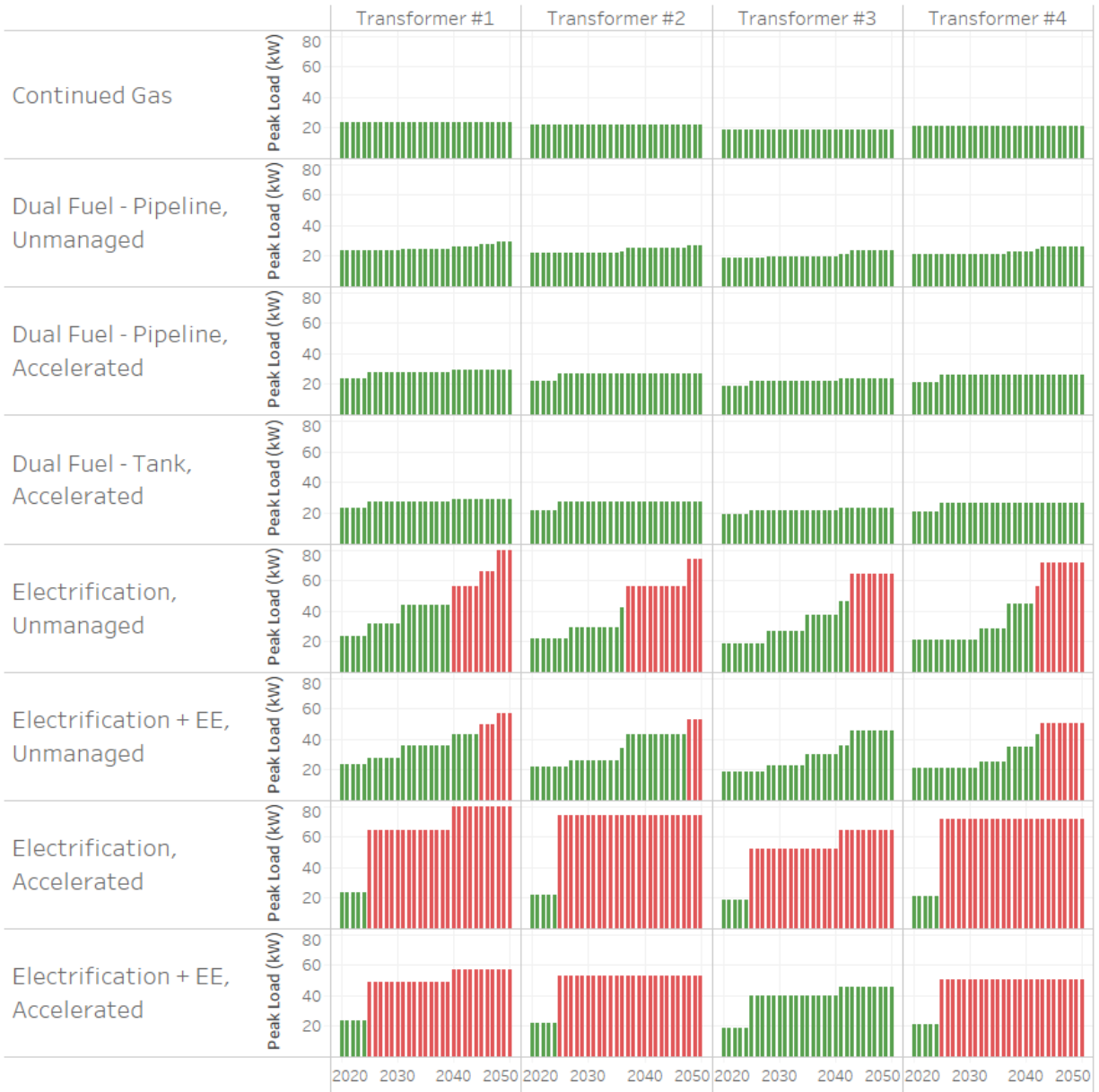
Figure 8. Peak loads for the single-family segment's four transformers under each scenario. Green represents peak load below the rated transformer capacity; red signifies the transformer capacity is exceeded.
