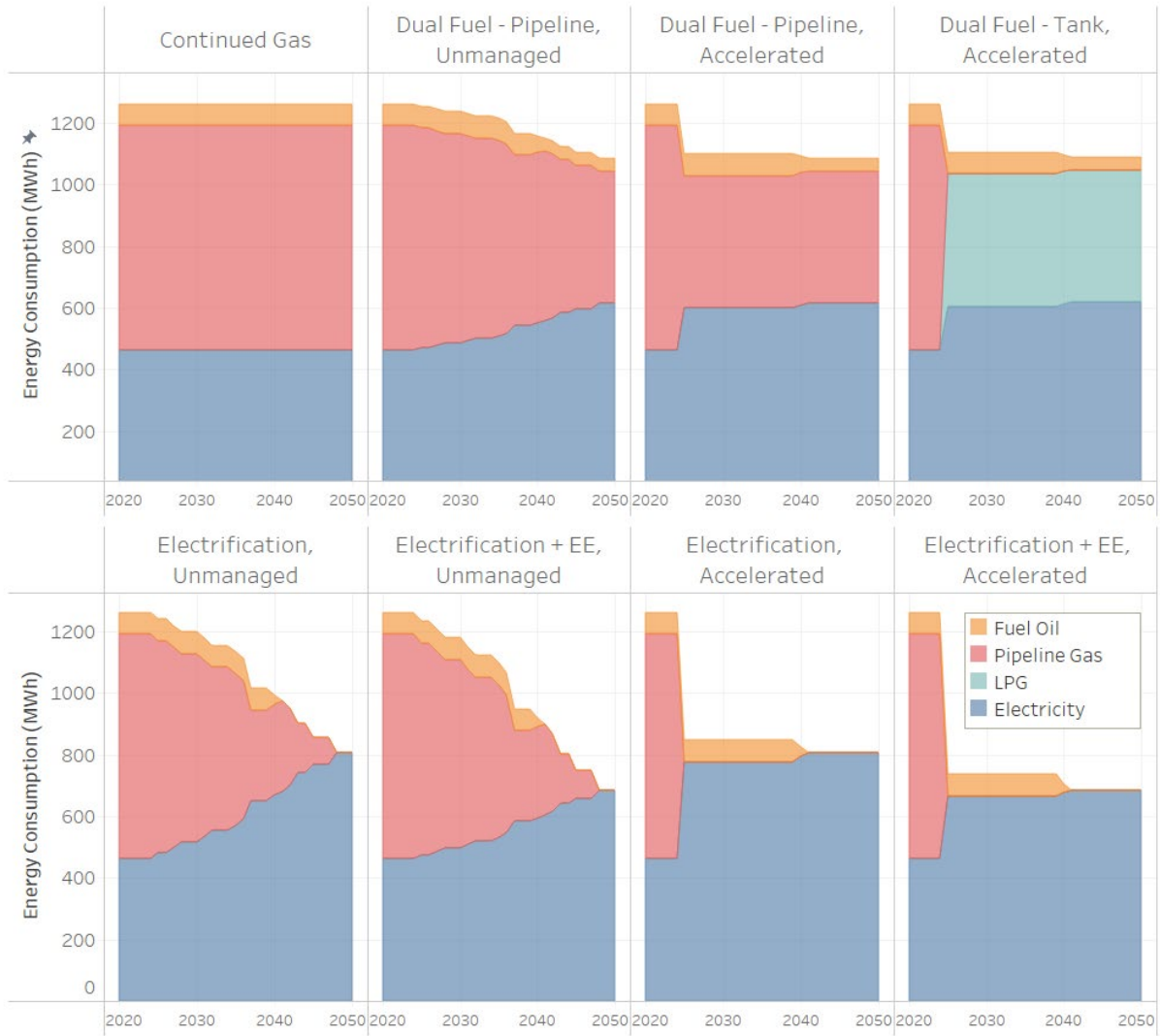
Figure 3. Total energy consumption by scenario for the single-family segment. “+ EE” scenarios indicate the addition of deep building efficiency measures to reduce total energy use and lower electric peak demand.
