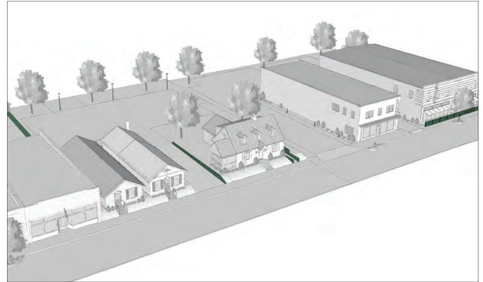
Fences and walls can be used to delineate front setback areas, to divide parking lots, as retaining walls at changes in grade, or as edges for ramps.
