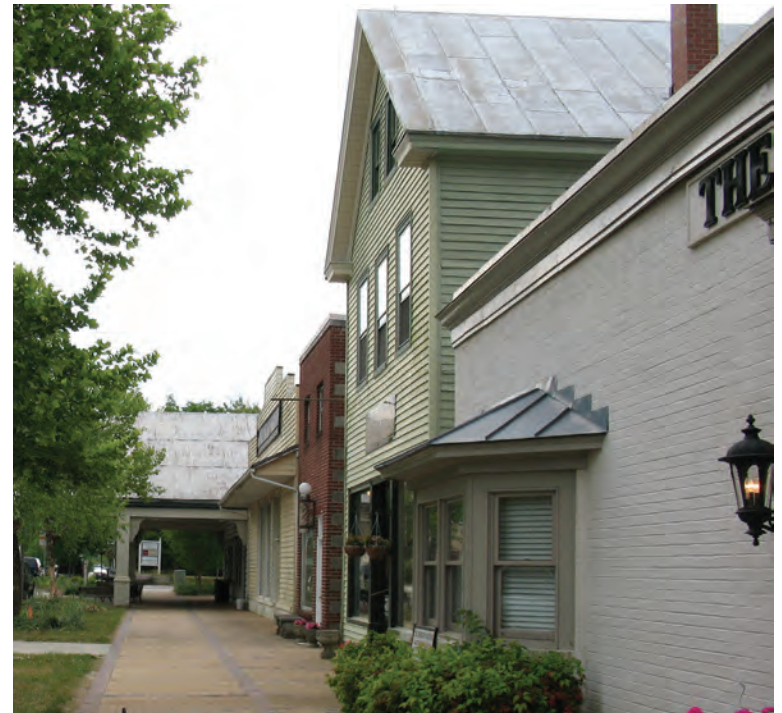
Common roof forms include a mix of flat roofs hidden by parapet walls, gables perpendicular to the street, and gable roofs parallel to the street.
