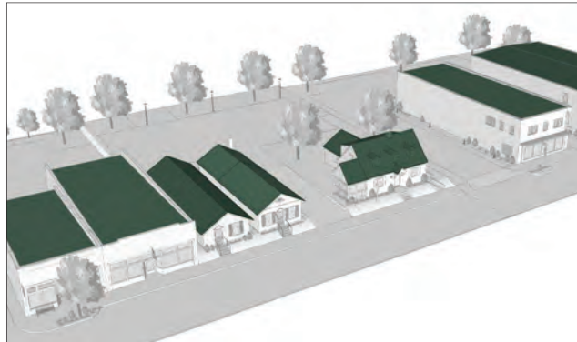
Common roof forms include a mix of flat roofs hidden by parapet walls, gables perpendicular to the street, and gable roofs parallel to the street.
