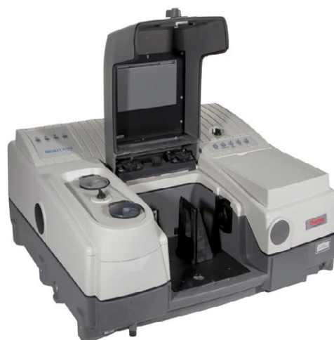
Fig. 1 Thermo Nicolet 4700 FTIR spectrometer. Note the standard size sampling compartment open featuring a simple transmission setup.
