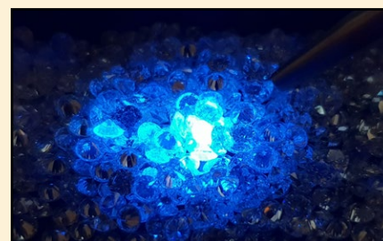
Fig. 6 Fluorescence emitted by natural diamonds illuminated by a high power UV probe. The most common color is blue but it is also possible to observe reactions such as yellow, yellow-green, pale whitish blue and pink.
