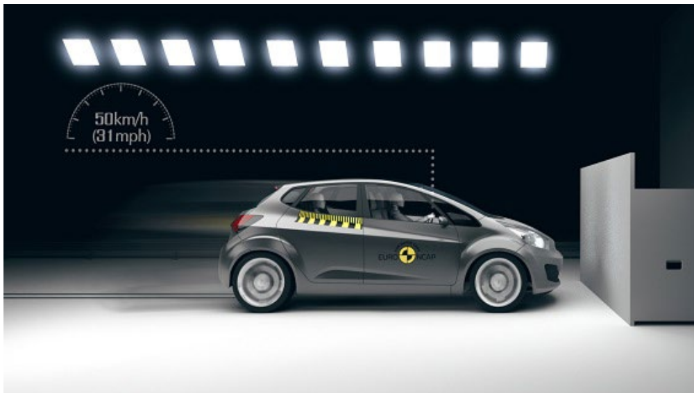
Figure 17 - EuroNCAP Full Width Rigid Barrier
