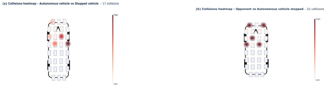
Figure 11 - Statistical weights for families of front-end involved impacts in autonomous vehicles in mixed traffic
