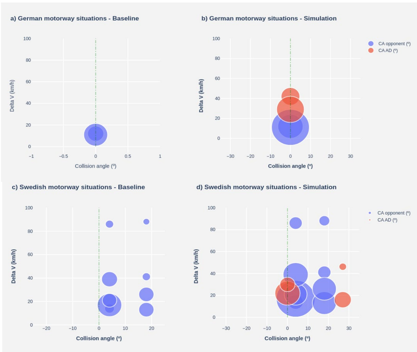
Figure 1 - Data visualisation of representative cases of motorway front-to-rear-end collisions: a) German motorway situations - Baseline and b) German motorway situations - Simulation, c) Swedish motorway situations - Baseline and d) Swedish motorway situations - Simulation (10)
