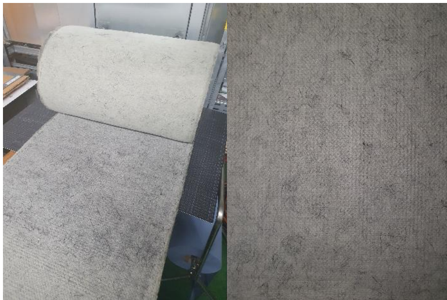
Figure 6: left: Continuous roll of nonwoven made from PA6, aramid and carbon fibers, right: Detailed representation of the random fiber orientation of the nonwoven
