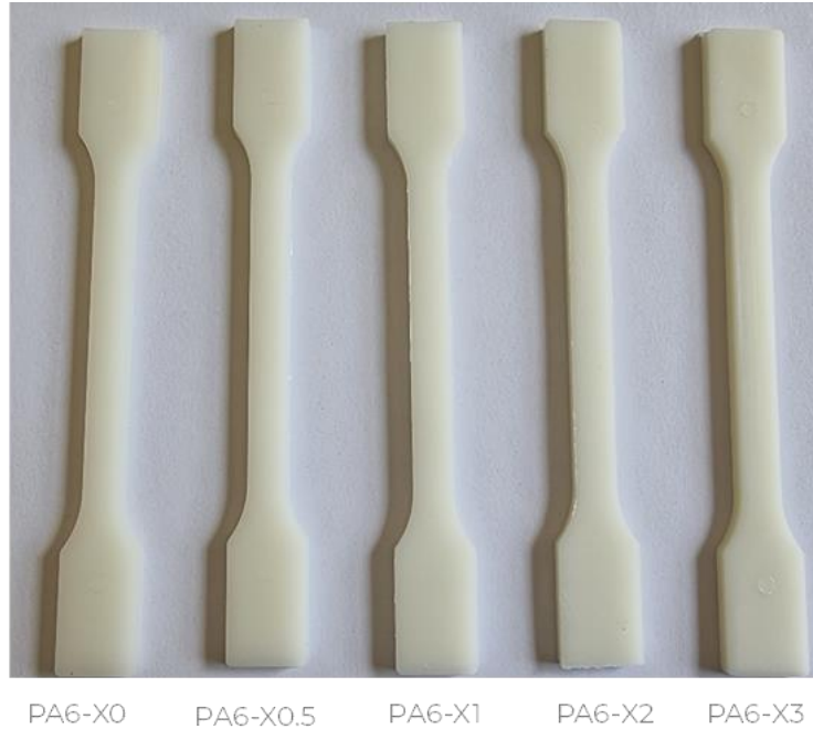
Figure 2: Tensile samples of polyamide 6 with different amounts impact modifiers
