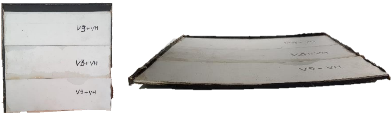
Figure 20. Hybrid laminates: result with the Vestamelt Hylink® Primer
