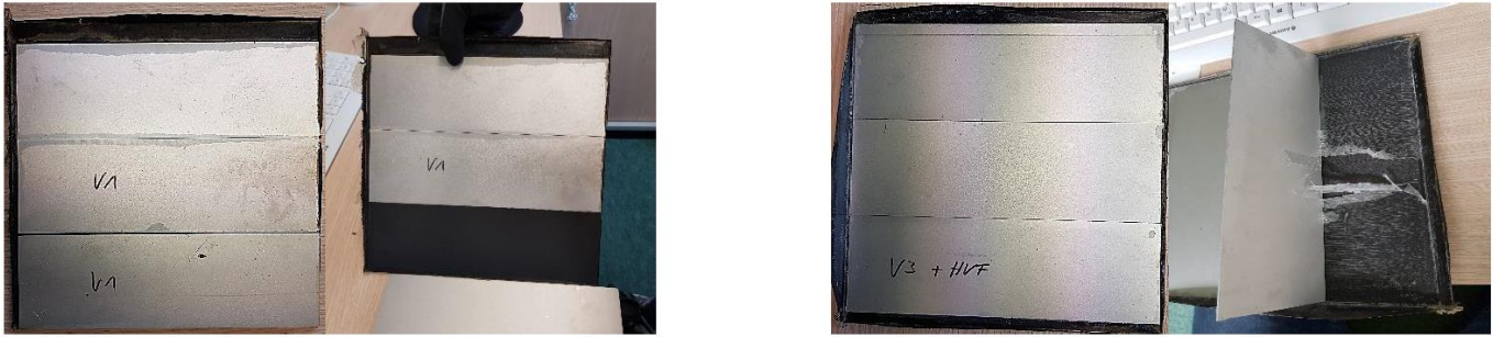
Figure 19. Hybrid laminates: without primer (left); with PP-MAH primer (right)
