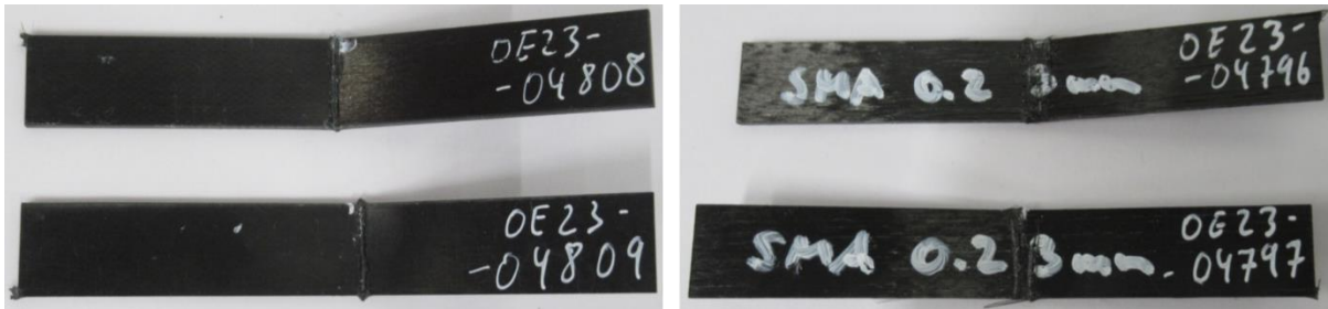
Figure 13. Examples of coupons after bending tests at RT. Left: variothermal process. Right: 3 mm spaced wires, placed at the top.
