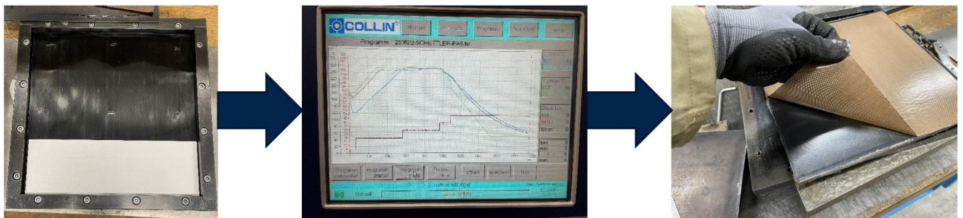
Figure 18. Preparation of laminates with hot press
