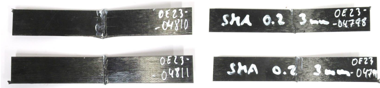
Figure 15. Examples of coupons after bending tests at 100°C. Left: variothermal process. Right: 3 mm spaced wires, placed at the top.
