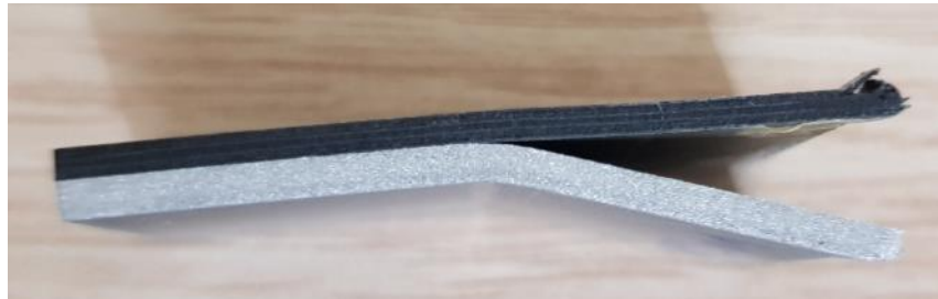
Figure 117: Tested specimen showing shear induced failure
