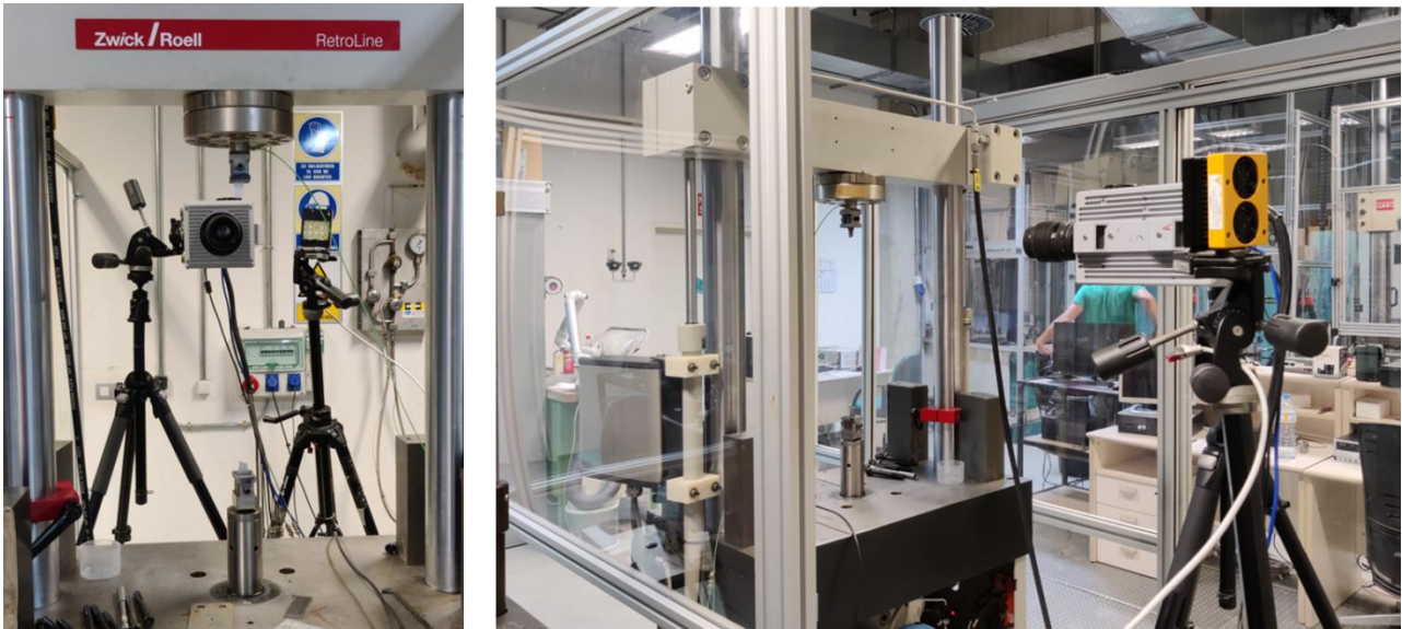
Figure 12: Front (left) and side (right) view of the testing equipment used for the dynamic tensile tests.
