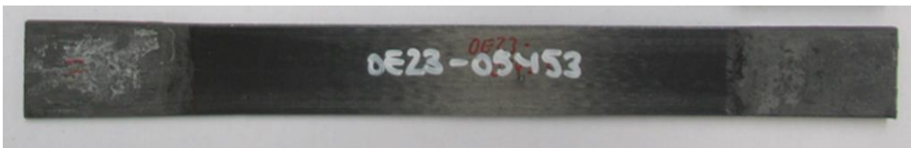
Figure 43: Coupon tested without tabs after test finished.
