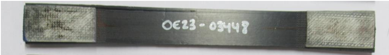
Figure 45: Coupon tested with milled tab ends after failure.
