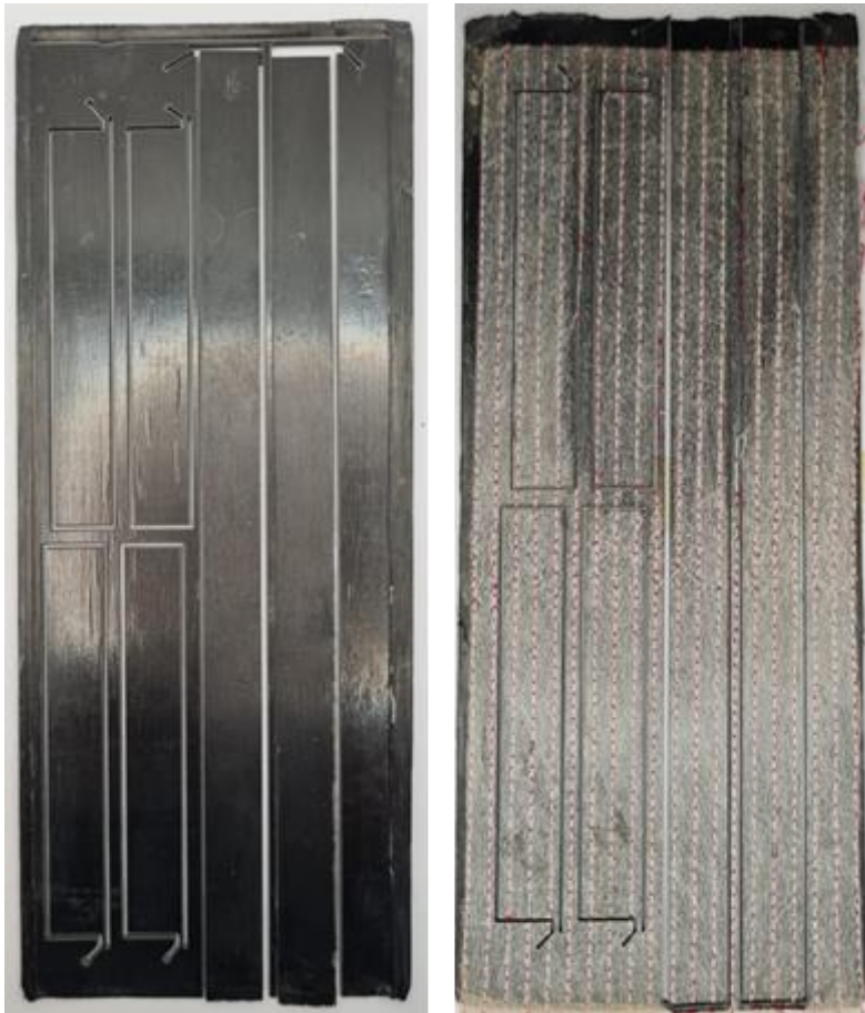
Figure 80: Cutted samples using waterjet technology placed in the origin plate
