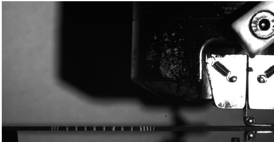
Figure 69: Test setup of interlaminar failure tests in Mode I with detail of the hinges employed.
