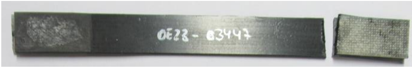
Figure 44: Coupon tested with sharp tabs after failure.
