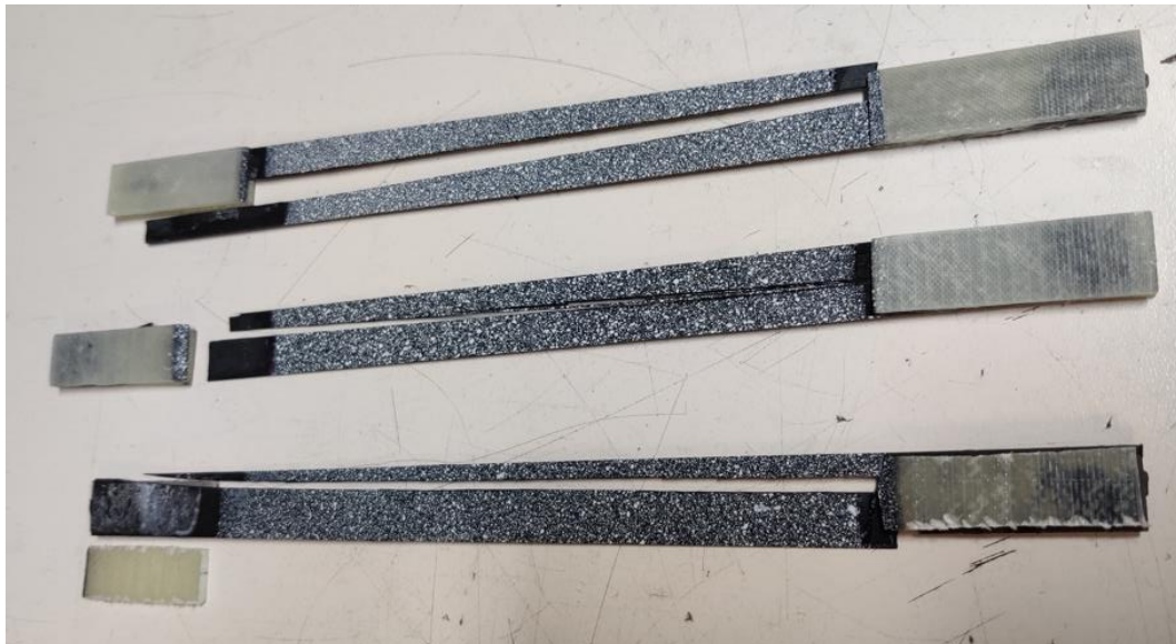
Figure 50: Aspect of the 0° coupons after dynamic tensile tests at 50s -1 .
