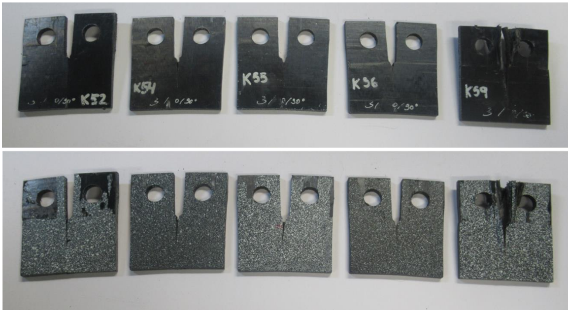
Figure 61: Aspect of CT coupons after testing.
