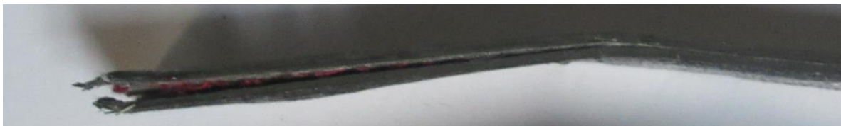
Figure 94: Delamination observed in the coupon with 200µm wires.
