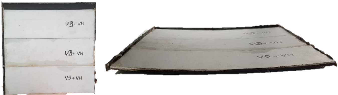
Figure 103: Hybrid laminates: result with the Vestmelt Hylink ® Primer
