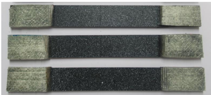
Figure 48: Aspect of the coupons (left) and force-displacement values from QS tests at 90° (right), for the thick coupons.
