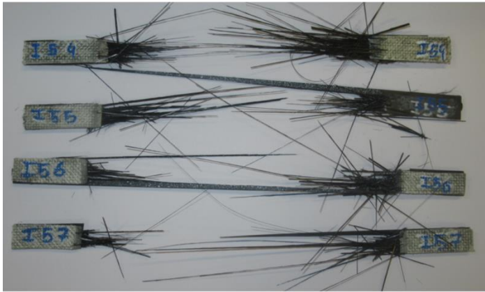
Figure 47: Aspect of the coupons (left) and force-displacement values from QS tests at 0° (right), for the thin coupons.
