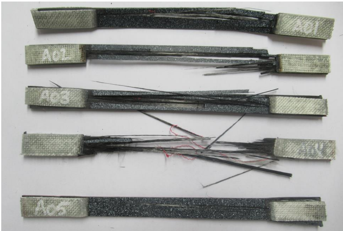
Figure 100: Aspect of SMA/CFRP coupons after QS tensile test.
