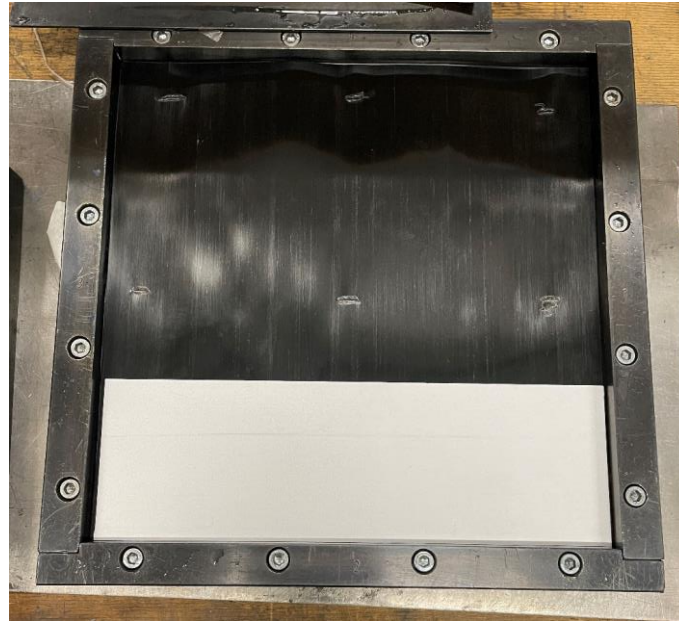
Figure 106: Placement of aluminum strips according to the last layer direction
