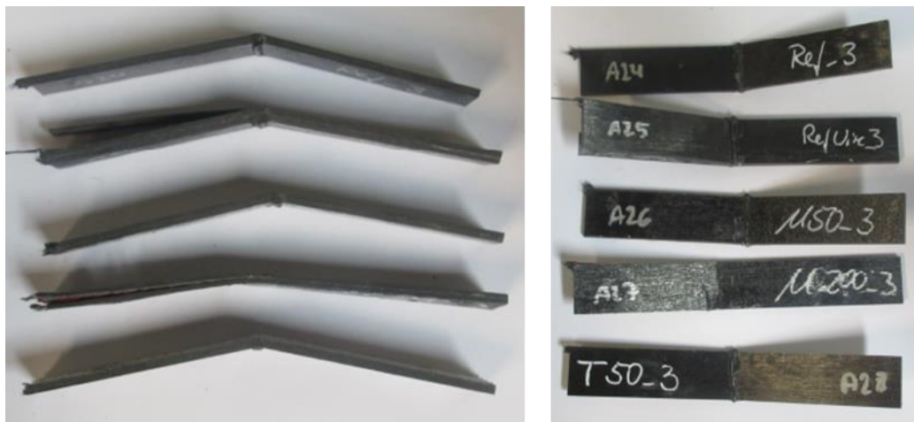
Figure 91: Aspect of SMA/CFRP coupons after three-point bending tests @ 100°C.
