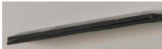
Figure 90: Early delamination observed in the coupon with 200µm wires.
