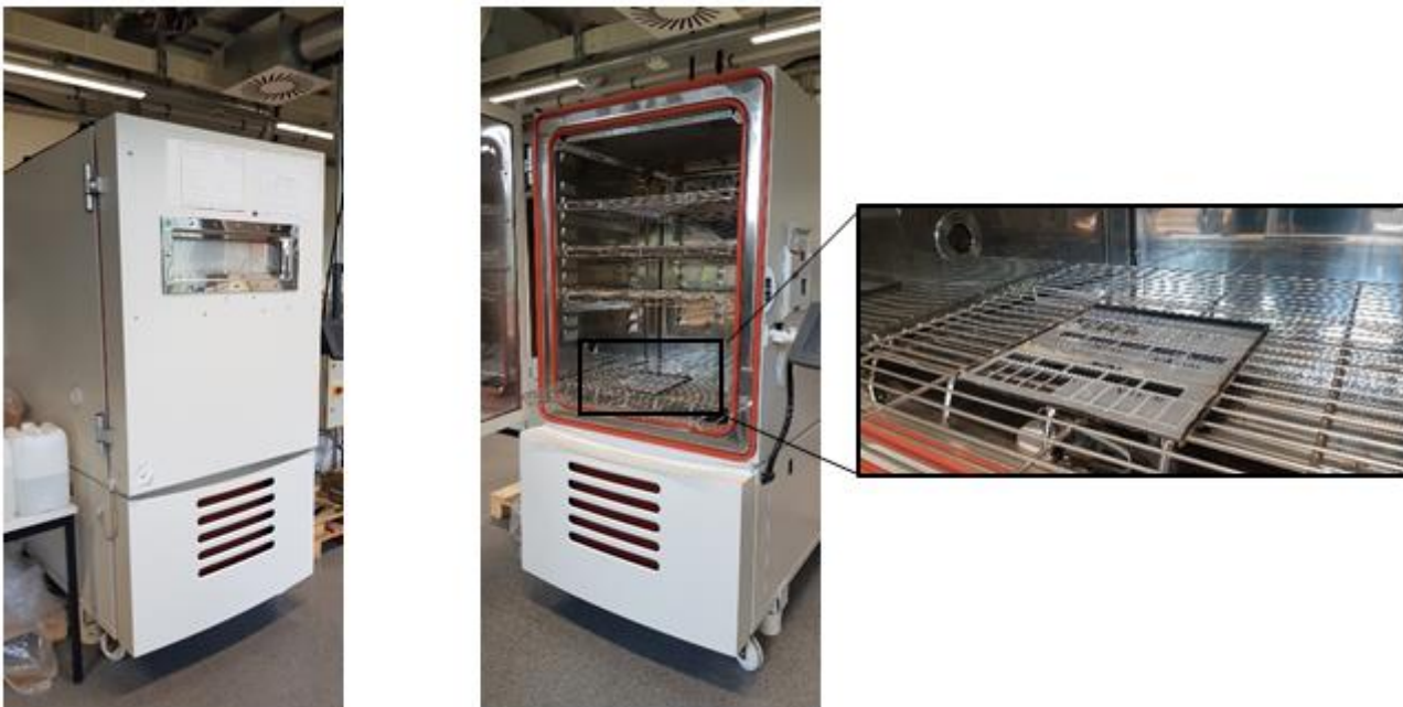
Figure 113. Climate chamber for carrying out climate change test as per PV1200
