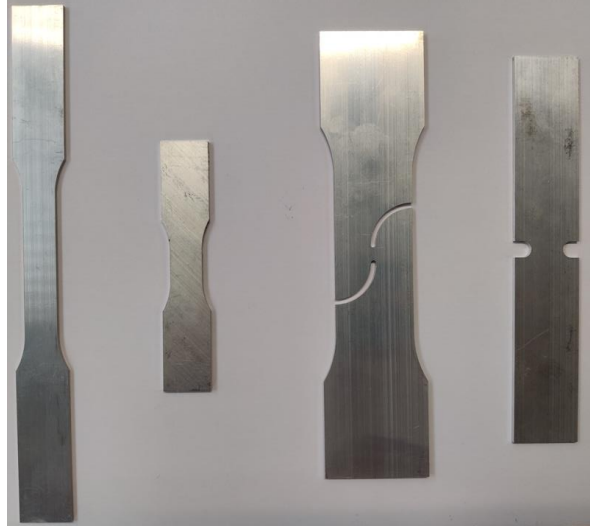
Figure 1: Examples of Al6063 coupons for testing. From left to right: QS tensile, dynamic tensile, shear and biaxial (small notch) coupons.
