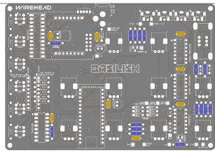
Place ceramic capacitors, solder all pins and trim all legs to 1-2mm length.
