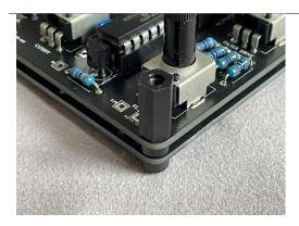
Once in place, attach a 12mm M3 nylon spacer to each screw
