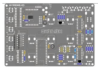
Place the transistor and voltage regulator.
