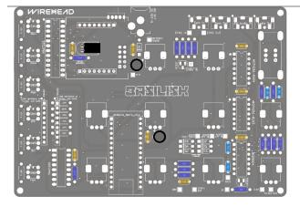
Place the 100uF electrolytic capacitors & solder all pins
