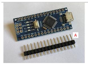
Insert the longer legs of the Arduino Nano (marked A) through the Nano's PCB holes.
