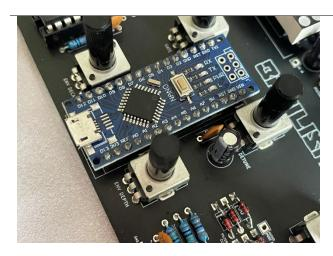
Insert the Arduino Nano V3 into the socket. Note this will be a firm fit so place one side into the socket then use both thumbs to apply even pressure and snap the Arduino fully into the socket.
