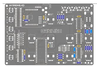
Place monolithic capacitors, solder all pins and trim all legs to 1-2mm length.
