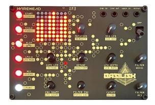
Place the front panel over all components, being careful to ensure the potentiometer, audio jacks, switches and LED matrix all fit through their respective holes
