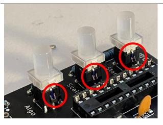
The coloured stripe on each switch which indicates the LED colour must be facing the INSIDE of the synth.
