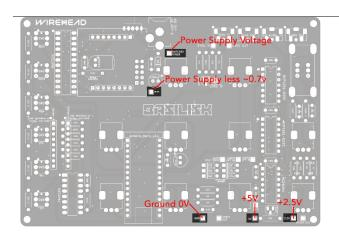
Using a multimeter with continuity mode, ensure there are no shorts between any of the power supply test points (GND, SWITCHED POWER, DC IN, 5V, 2.5V).
