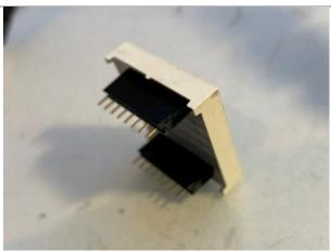
Insert the LED matrix into the 1x8 headers then loosely place into the sockets on the PCB
