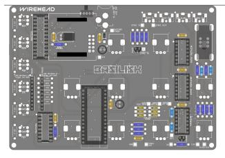
Keeping the front panel and LED matrix in place, solder pins 1 and 8 of both header sockets.
