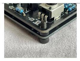
Place the main PCB onto the screws & washers
