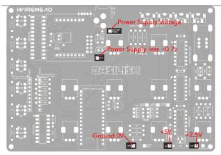
The Basilisk uses the Arduino's 5V voltage regulator to generate 5V.
