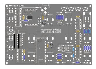
Place the resistor arrays.
