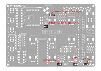
Disconnect the USB cable, connect 9-12V DC to the power jack and turn the power switch on
