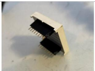
Insert the LED matrix into the 1x8 headers then loosely place into the sockets on the PCB
