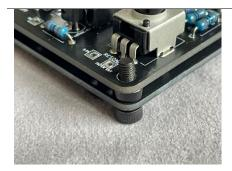
Place the main PCB onto the screws & washers
