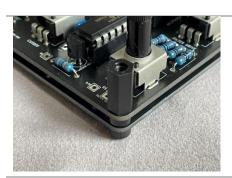
Once in place, attach a 12mm M3 nylon spacer to each screw
