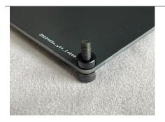
For each mounting hole in the rear panel insert a 10mm-long hex screw through from the underside of the rear panel then attach an M3 washer
