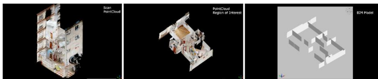
Figure 1: Application of automatic Scan-To-BIM tool in the Spanish Demo Case. The first and second images represent the point clouds of the Demo Case and of the Region of Interest (one apartment). The third image represents the preliminary BIM model of the Region of Interest.
