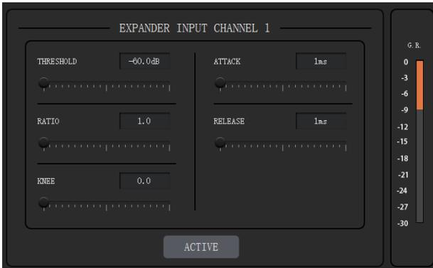
**THRESHOLD:** The signal below will be identified as noise and attenuated, with a range of [-60.0, 0.0] dB.
