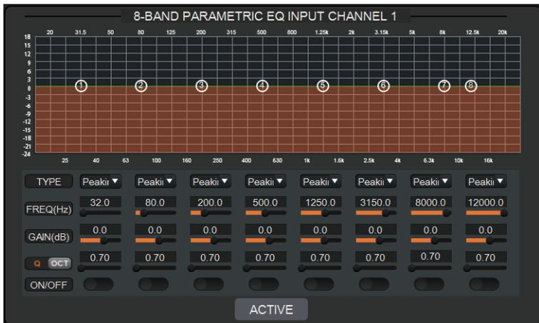
**TYPE:** Provides 5 types of band/filter, with H-Pass, L-Pass, H-Shelf, L-Shelf and Peaking optional.
