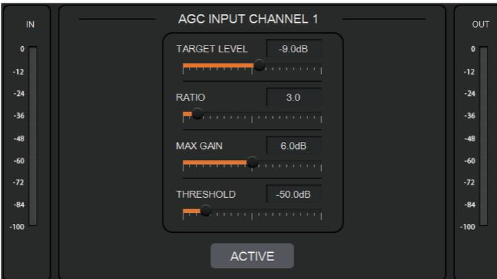
**TARGET LEVEL:** The desired output signal level, with a scale of [-20.0, 0.0] dB.
