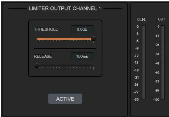
**THRESHOLD:** Shows that level signals above threshold will be attenuated, with a scale of [-60.0, 0.0] dB.
