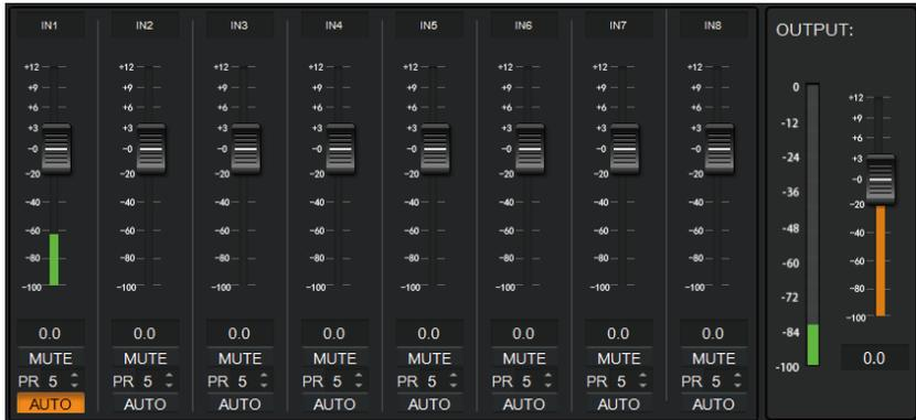
**AUTO:** Click AUTO to add the corresponding input MIC to the auto mixing system. Then you can use the fader of the MIC input channel to adjust its signal level for controlling the mixed volume on the input channel, or click MUTE to mute the MIC input channel.
