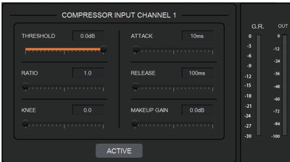
**THRESHOLD:** The level that the signal above it will be compressed, with a scale of [-60.0, 0.0]dB.
