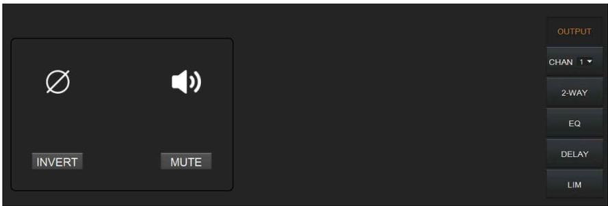
**INVERT:** When pressed, inverts the polarity of the signal on the channel.
