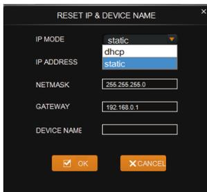
Select “dhcp” in the IP mode drop-down menu to select the dynamic DHCP mode. Then click “OK” to use DHCP mode for the network.
