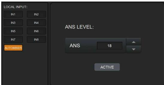
**LOCAL INPUT:** The source input channels. You can select the channel based on actual access conditions. AUTOMIXER refers to mixed signals after the AUTOMIXER process.
