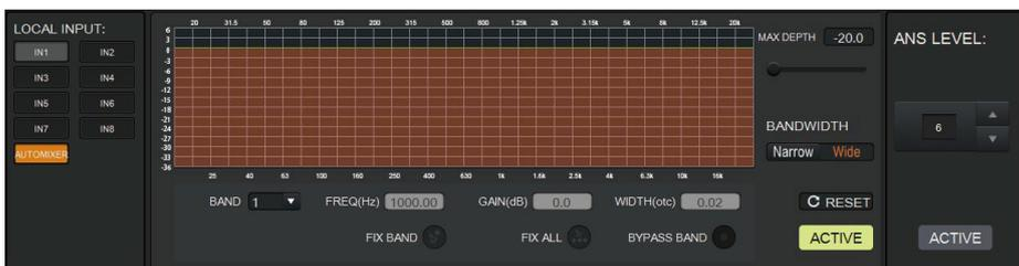
**LOCAL INPUT:** The source input channels. You can select the channel based on actual access conditions. AUTOMIXER refers to mixed signals after the AUTOMIXER process.
