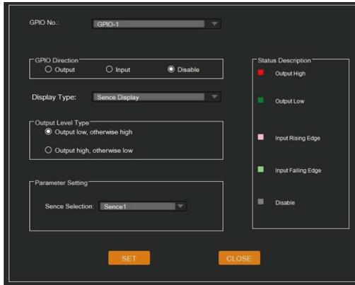
You can set the GPIO function as needed, see details at GPIO Setting page. You can also check GPIO status by GPIO LED at the top-right corner of Host page.
