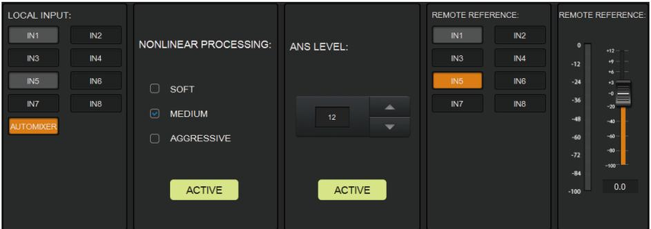
**LOCAL INPUT:** The source input channels. You can select the channel based on actual access conditions. AUTOMIXER refers to mixed signals after the AUTOMIXER process.
