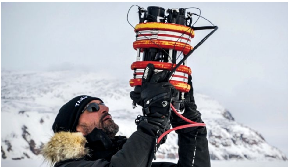
Photo 9.3: The author holding an instrument designed for light measurements under sea ice. Here he exposes it to sky light for quality control of the sensors.
