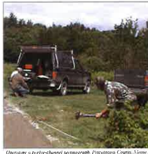
Operating a twelve-channel seismograph, Piscataquis County, Maine.
