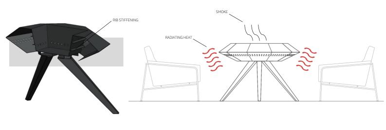
Unlike conventional firepits, the internal liner design takes advantage of rib stiffening used to prevent distortion due to heat, as seen above in the cross-sectional view.
