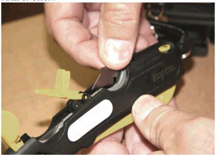
**BLADE STORAGE/STORAGE LID:** Make sure blades are flush with carriage as shown below. Close lid, blades must not interfere with lid closing.
