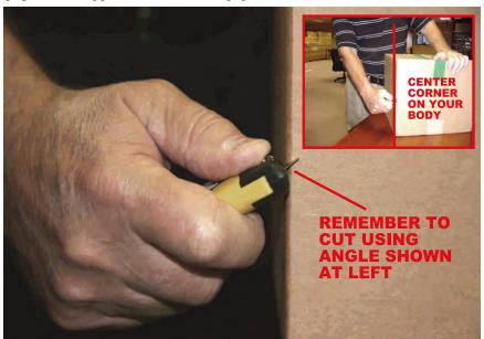
**TOP CUT:** Extend the edge guide. Using the proper cutting angle. Center box in front of you as show on inset picture. Engage blade and make cut. Relax your grip on the trigger once blade is engage in the box.
