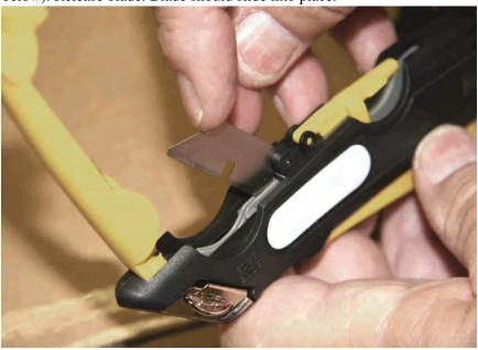
**CHANGING BLADE/CLOSING CARRIAGE COVER:** Make Sure blade is flush with carriage as shown below. Close cover, blade must not interfere with cover closing. If cover does not close easily repeat above procedure.
