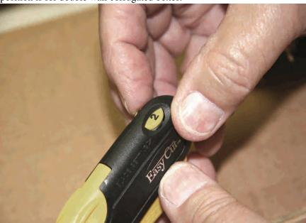
**SETTING THE BLADE DEPTH (3):** Push down and rotate blade depth dial to desired position. You should feel the dial click into place. Position (3) is used for extra thick boxes.
