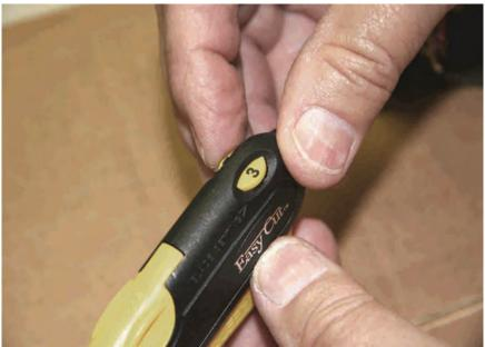
**LOCKING THE BLADE** (L): Push down and rotate blade depth dial to locked position. You should feel the dial click into place. This locks the blade inside the cutter.
