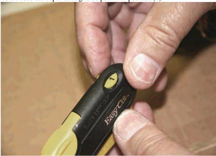
**SETTING THE BLADE DEPTH (2):** Push down and rotate blade depth dial to desired position. You should feel the dial click into place. The (2) position is for double wall corrugated boxes.
