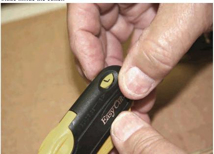
**CUTTER POSTURE:** IMPORTANT. Shown below is the correct way to hold the cutter when cutting. Squeeze the trigger to engage blade. Once blade is engaged into box, relax your grip on the trigger.
