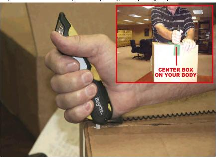
**CENTER CUT:** Center box in front of you as show on inset picture. Use the flat part of the cutter to establish the proper cutting angle. Never cut at 90° as shown on previous page. Engage blade and make cut. Relax your grip on the trigger once blade is engaged in the box.
