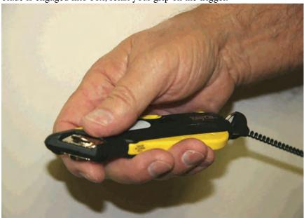
**CUTTER POSTURE:** When using the edge guide, place your thumb on the top of the edge guide. This is the correct way to hold the cutter for making top cuts. There are two ways to get the edge guides out shown on next page.
