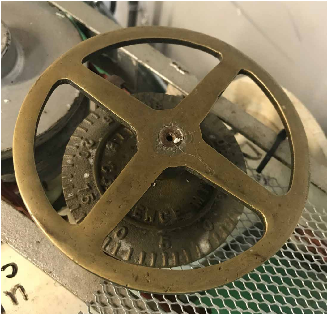
Figure 2: The hand wheel on the vertical shaft has a threaded connection to the supporting leverage system. A dial is calibrated in 0.001" vertical movement between roll and plate.
