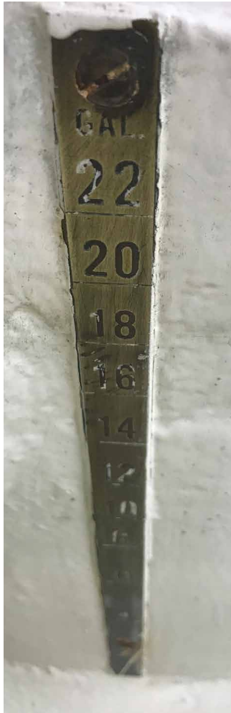
Figure 1: The tub is calibrated in pounds of water to facilitate loading.
