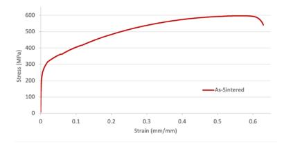
All data represents samples with 15 mm printed and 13 mm sintered thickness, sintered using a standard cycle in Rapidia's F2 Vacuum Furnace. Tensile testing and hardness and density measurements were performed at an accredited third party laboratory. Corrosion resistance and metallography were studied in-house at Rapidia. Note that material performance is influenced by numerous factors such as print quality, furnace loading, and part thickness and geometry.
