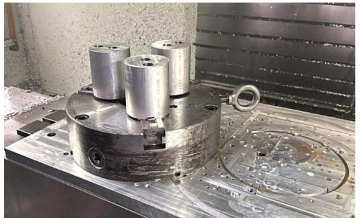
The lathe chuck on the CNC mill as a fixture
