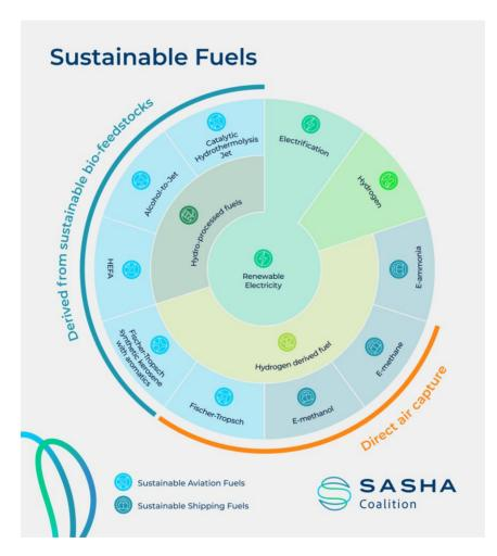
This graphic shows the different potential fuel production pathways for the aviation and shipping sectors. Other than where direct electrification can be used, hydrogen is required either as a key component of these fuels or as part of their processing.
