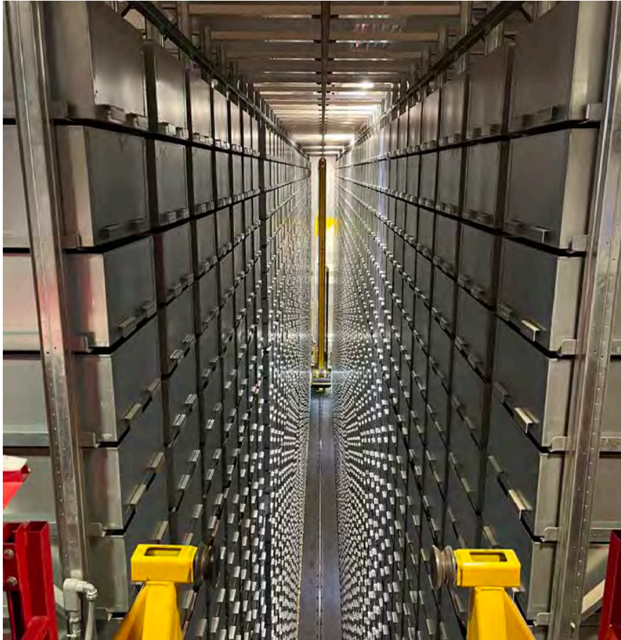
Above: A row of shelved storage inside the automated storage and retrieval system Opposite page: Rain garden reading lounge
