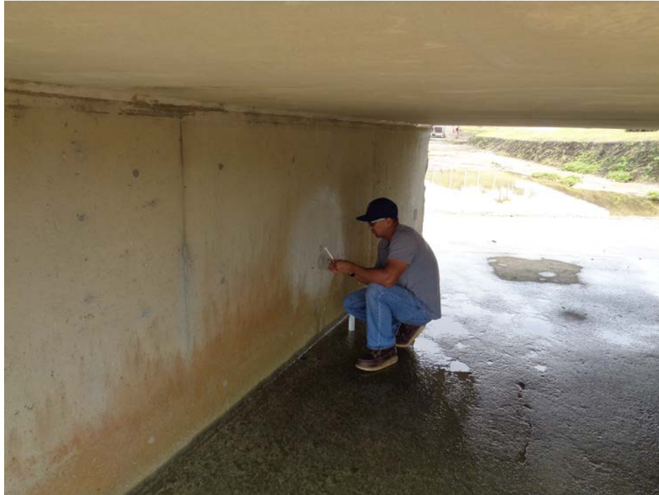
Figure 6 – Collecting rilem test tube, white area where Surtreat system applied
