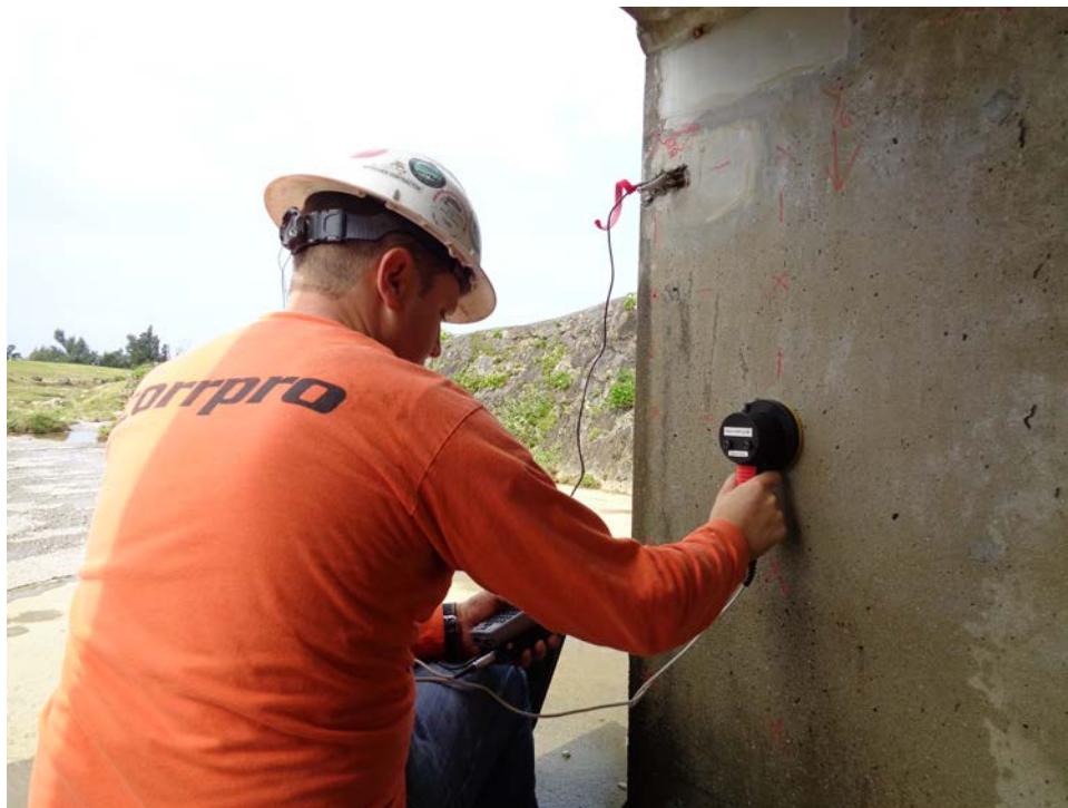
Figure 5 – Measuring corrosion rate
