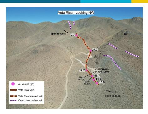
Drone photo looking northwest showing 700 m strike length of Veta Rica, select surface rock chip samples and established drill pads. The Veta Rica vein remains open to both the west and, in the foreground, to the east where it passes under shallow cover.
