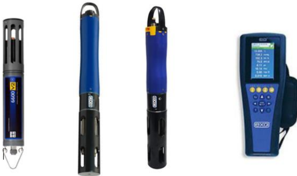
Figure 2. YSI 6600 V2 multiparameter data sonde (left), YSI EXO2 multiparameter data sonde (second to the left), YSI EXO3 multiparameter sonde (second to right), and YSI 650 MDS Handheld (right). Source: YSI
