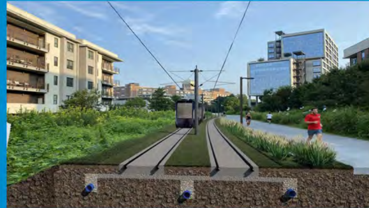
Embedded Slab Track with Grass Edges
