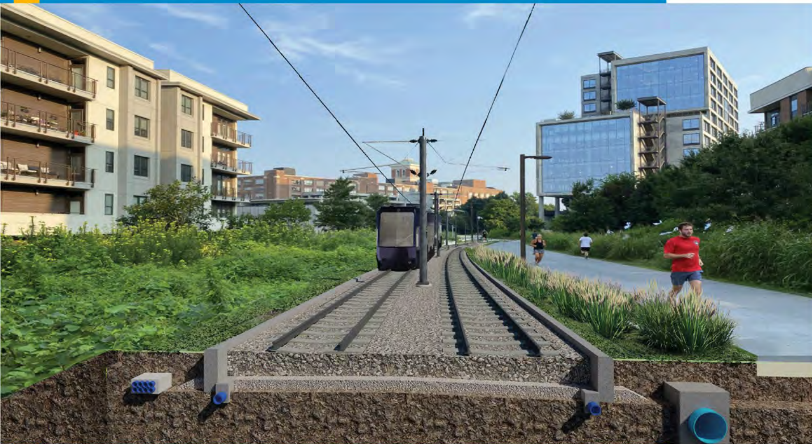
Retained Ballast Track with Maximized Green Space
