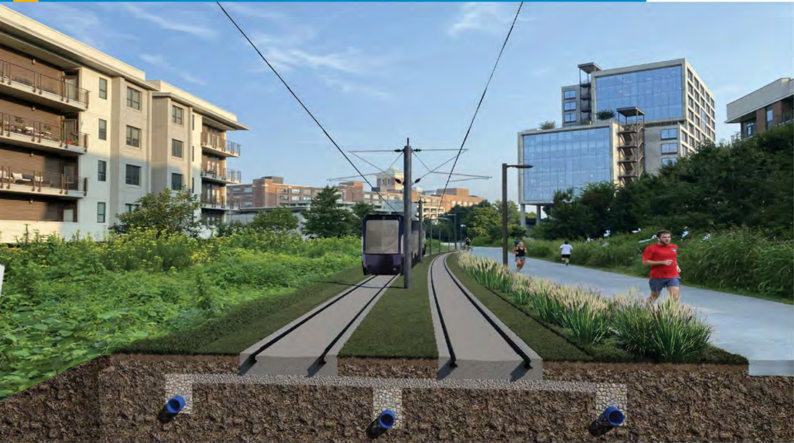
Embedded Slab Track with Grass Edges
