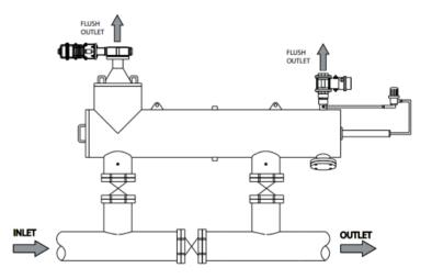
Specifications: Standard filters are from AISI 304. Internal parts are from AISI 316L. Standard filters are rated to 150 psi and 160°F
