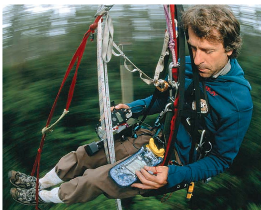
Figure 3. Ecologist Roman Dial collecting canopy element data in a 250-foot tall Eucalyptus forest in Australia. Dial is suspended by a vertical transect rope as he collects and records data using a waterproof PDA. The PDA is connected to a digital compass and digital laser range finder. These surveying instruments automatically download location measurements into the PDA while Dial uses the PDA's handwriting recognition software to record the located object's identity. (Photo courtesy of Bill Hatcher Photography.)
