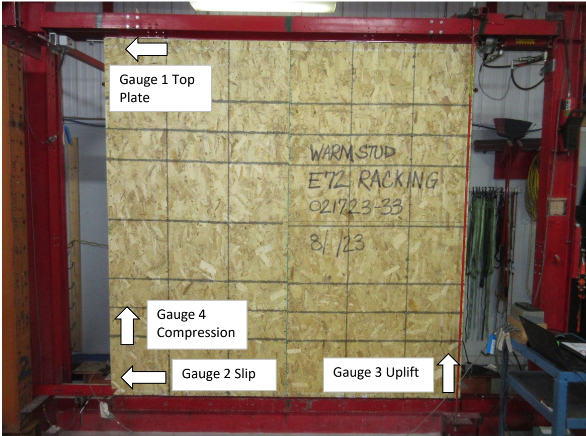
Typical Test Setup (Arrows indicate positive deflection, per ASTM E72-22)
