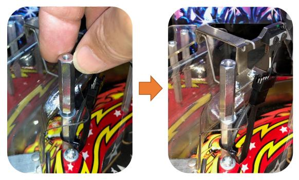
k) Before installing the KISS Target Nano Topper, loosen the screw of the stainless steel mounting bracket and rotate the mounting bracket to suit your desired position as shown below. <u>TIP</u>: To position the Nano Topper close to the left side of the cabinet, rotate the bracket position as shown in the 3<sup>rd</sup> or 4<sup>th</sup> picture shown below and tighten the screw, but <u>DO NOT OVER TIGHTEN!</u> The choice is YOURS.
