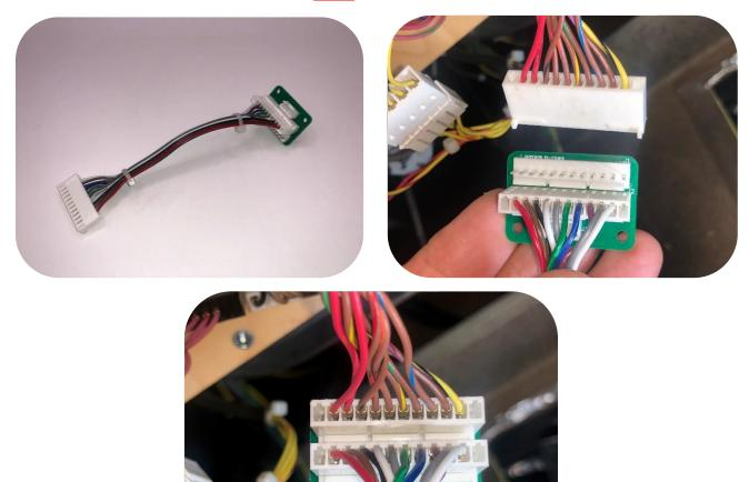
r) Take the pre-connected cable which is connected from the J2 socket of the Lamp Board Splitter board and route the unconnected end back to the CN8 socket of the Node Board 11 as shown below:
