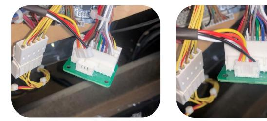
t) Using the supplied white cable tie, tie the cables from Lamp Board Splitter board to an existing fixed wiring loom securely as show below:
