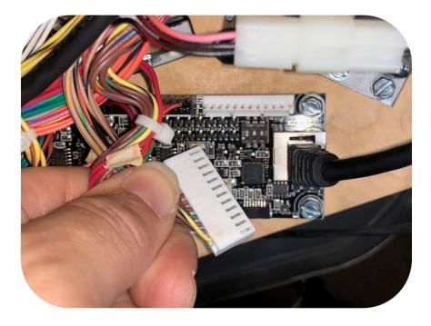
q) Connect the playfield CN8 cable into the <u>J1 socket</u> of the Lamp Board Splitter board as shown below. NOTE: The CN8 connector can <u>ONLY</u> be inserted one way as shown.
