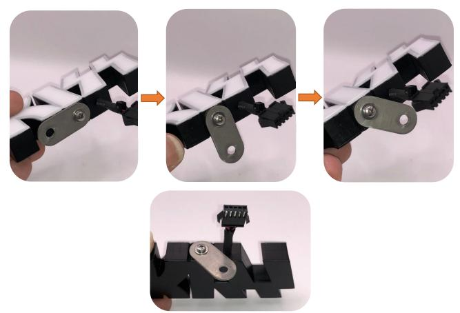
Connect the KISS Target Nano Topper <u>female</u> 5 pin connector to the <u>male</u> 5 pin connector Lamp Board Splitter connection cable, note to align the notch of both connectors as shown below. The connector can only be connected one way.
