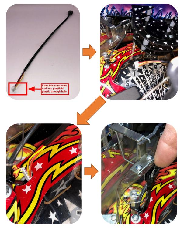
j) Screw the Aluminium 1 <sup>1</sup>/<sub>2</sub>" Hex Spacer 6/32" mount through the supplied metal washer onto the LEFT PLASTIC RAMP TOP FLAP firmly with your hand or use a hex tool, but <u>DO NOT OVER TIGHTEN!</u>
