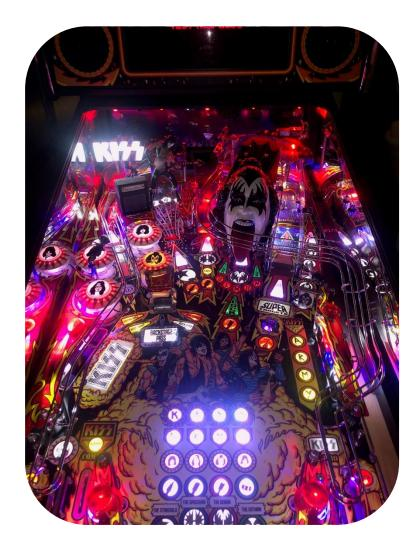
b) Alternatively, to test each K, I, S, and S letters of the topper individually, navigate to the DIAGNOSTIC MENU > SINGLE LED TEST and select each LED number from 67 (K), 68 (I), 69 (S) and 70 (S) are lit individually as shown below:
