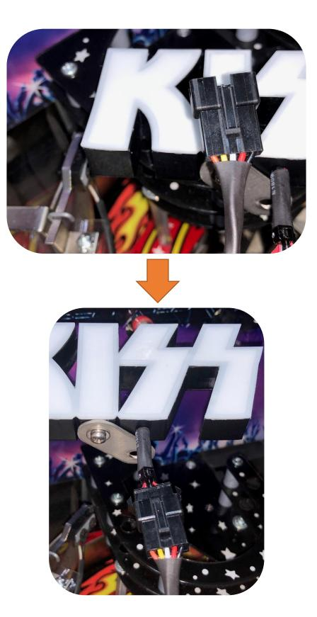
m) Attach the KISS Target Nano Topper with its steel bracket to the Aluminium 1 ½" Hex Spacer and use the original metal screw and washer from step 2(h) to tighten and fix in place. Position topper as desired.
