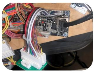
s) Connect the unconnected end (J3 cable connector end) of the Kiss Target Nano Topper cable that was inserted from above the playfield in STEP 2(i) and connect this into J3 socket of the Lamp Board Splitter board.
