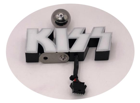
g) Unscrew the mounting metal top screw and washer situated on LEFT PLASTIC RAMP top flap exit in the TOP LEFT UPPER CORNER PLAYFIELD (i.e. next to the Paul Stanley figure) as shown below:
