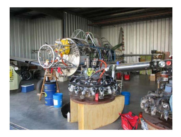
In this photo, we're cleaning out and replacing all the flex lines for the oil system and transferring all the parts from the old engine to the new one. The engine baffles were inspected and 3 of them had to be replaced due to corrosion, the prop governor was sent out & rebuilt and all related hardware was replaced. Lots of stuff going on in a small hangar!
