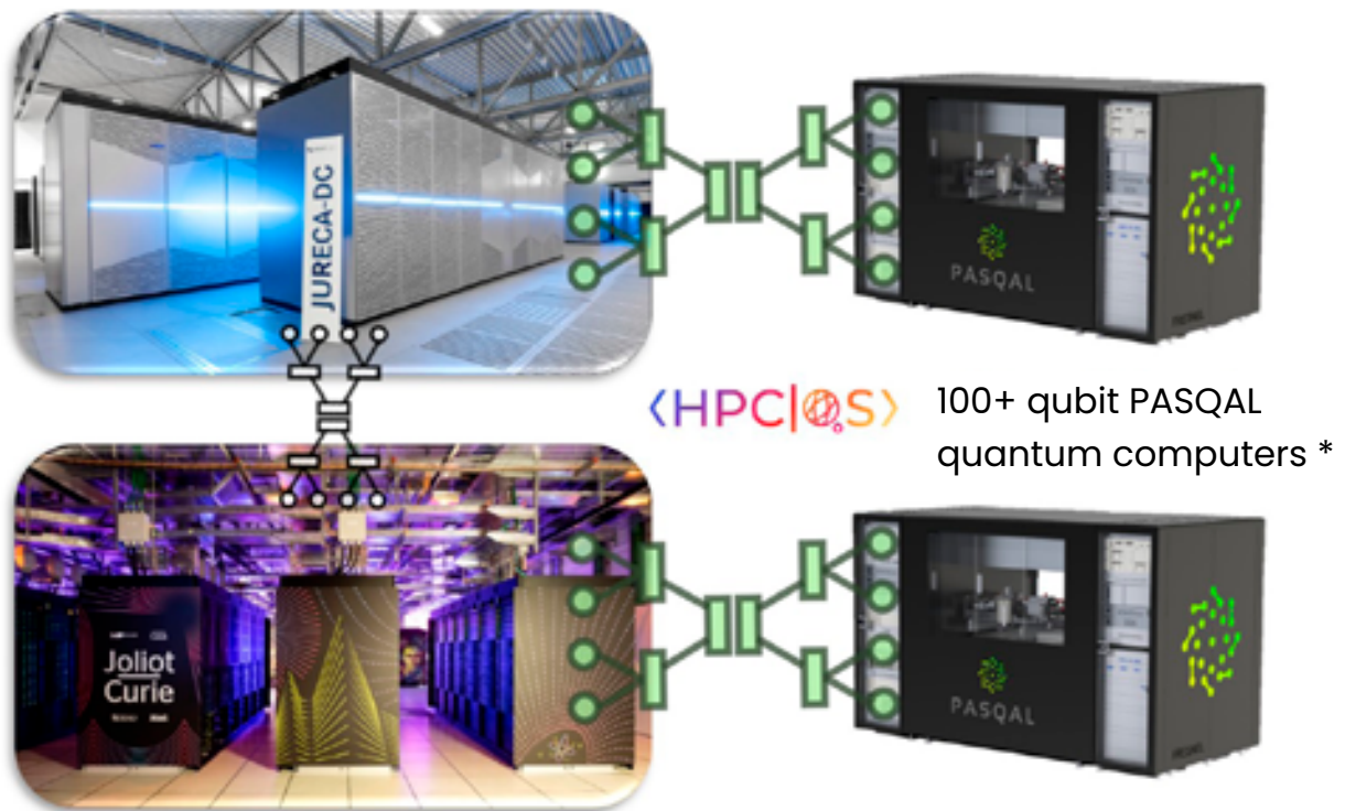
Fig.5. Integration of the PASQAL computers with the JURECA DC and the Joliot Curie supercomputers at FZJ and GENCI/CEA, respectively, as part of the HPCQS project * referred to as quantum simulators according to quantum flagship terminology
