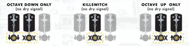
In **AUXILIARY MODE**, the middle key sends signal to the device placed in the loop. Achieve an OCTAVE UP or DOWN in parallel with that device by pressing the middle key and octave keys.
