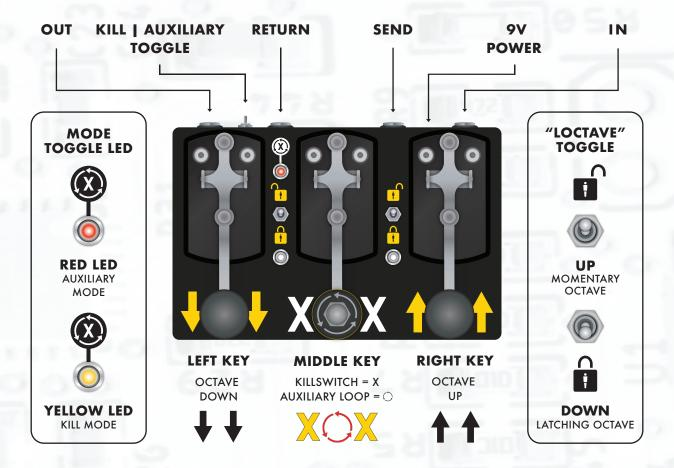
POWER CONSUMPTION: 250mA @ 9V | IN/OUT & SEND/RETURN: 1/4-inch Inst.Cable
