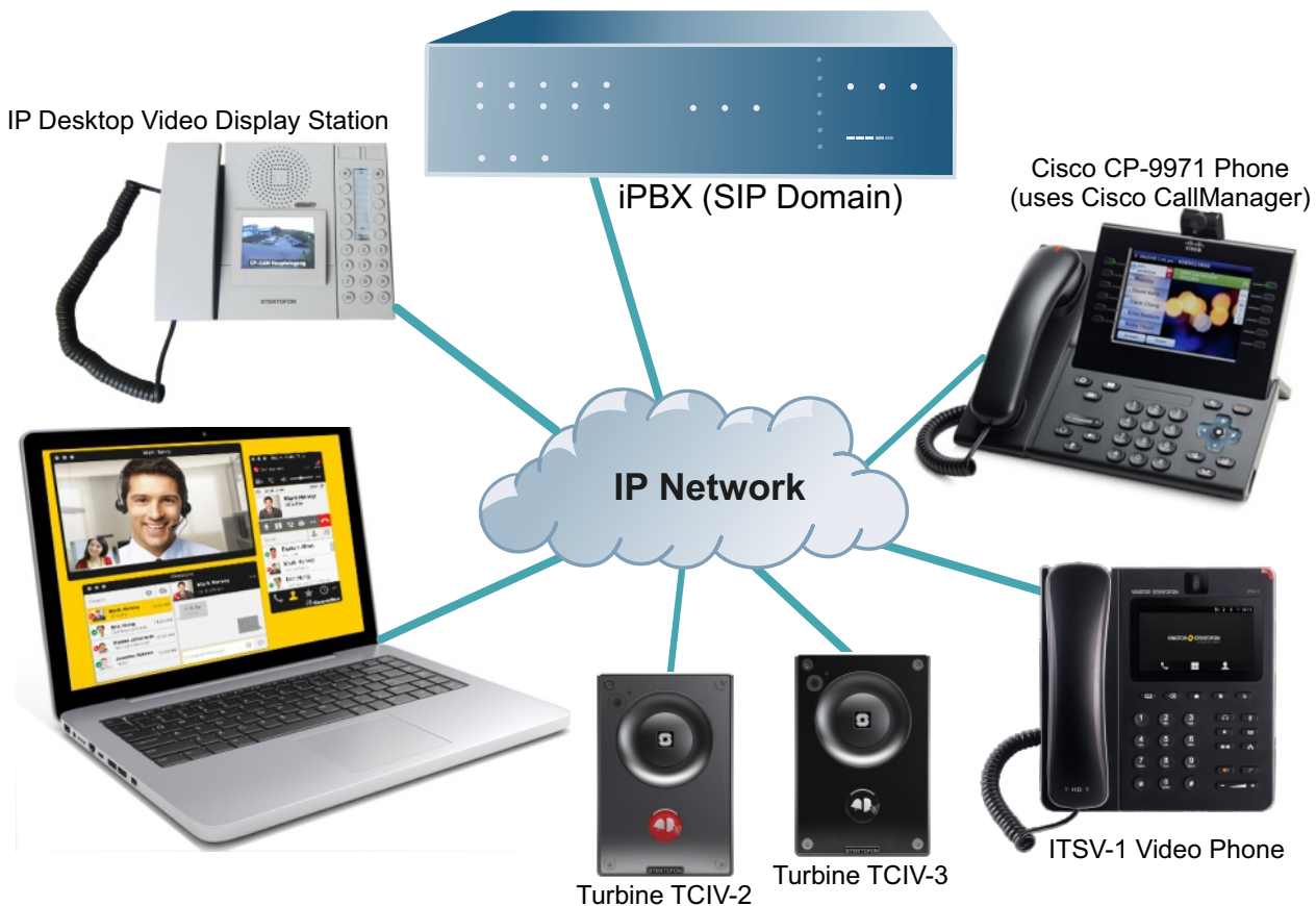
Figure 6 SIP Video Intercom System
