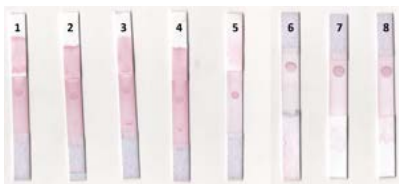
Figure 1: Lateral flow tests of SEA samples (1 ng/ \mu L) as well as BSA (1 mg/mL) and BB samples. In order from 1 to 4, the strips correspond to the test formats Apt5-AuNPs + Apt1/Apt2/Apt3/Apt4. Strip 5 corresponds to the BB-only solution while strips 6-8 correspond to the BB samples.
