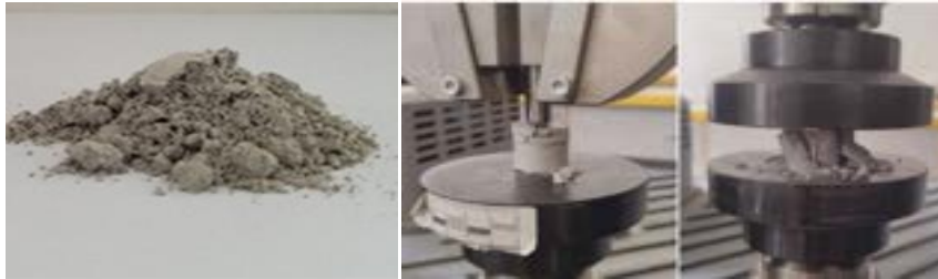
Figure 1: Original WCF grains (left) and indentation of hardened samples using a conically-shaped steel indenter forced into a sample (middle) and the uniaxial compression test (right), taken and adapted from (Kliková et al., 2025)
