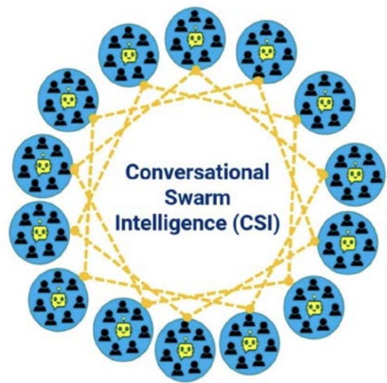
Fig. 1. Architecture for a Conversational Swarm Intelligence with AI agents assigned to each subgroup for passing and receiving conversational content.
