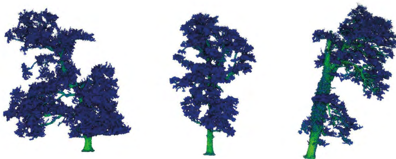
Figure 1: A 3D point cloud of storm damaged oak (crown damaged) acquired using a GeoSLAM ZEB Horizon LiDAR scanner.
