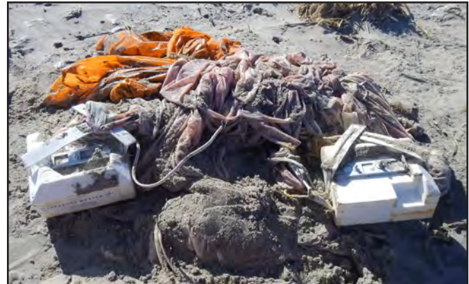
Figure 50: This weather balloon found on Cedar Island consisted of two instrument boxes, cotton string, latex balloon and plastic parachute.
