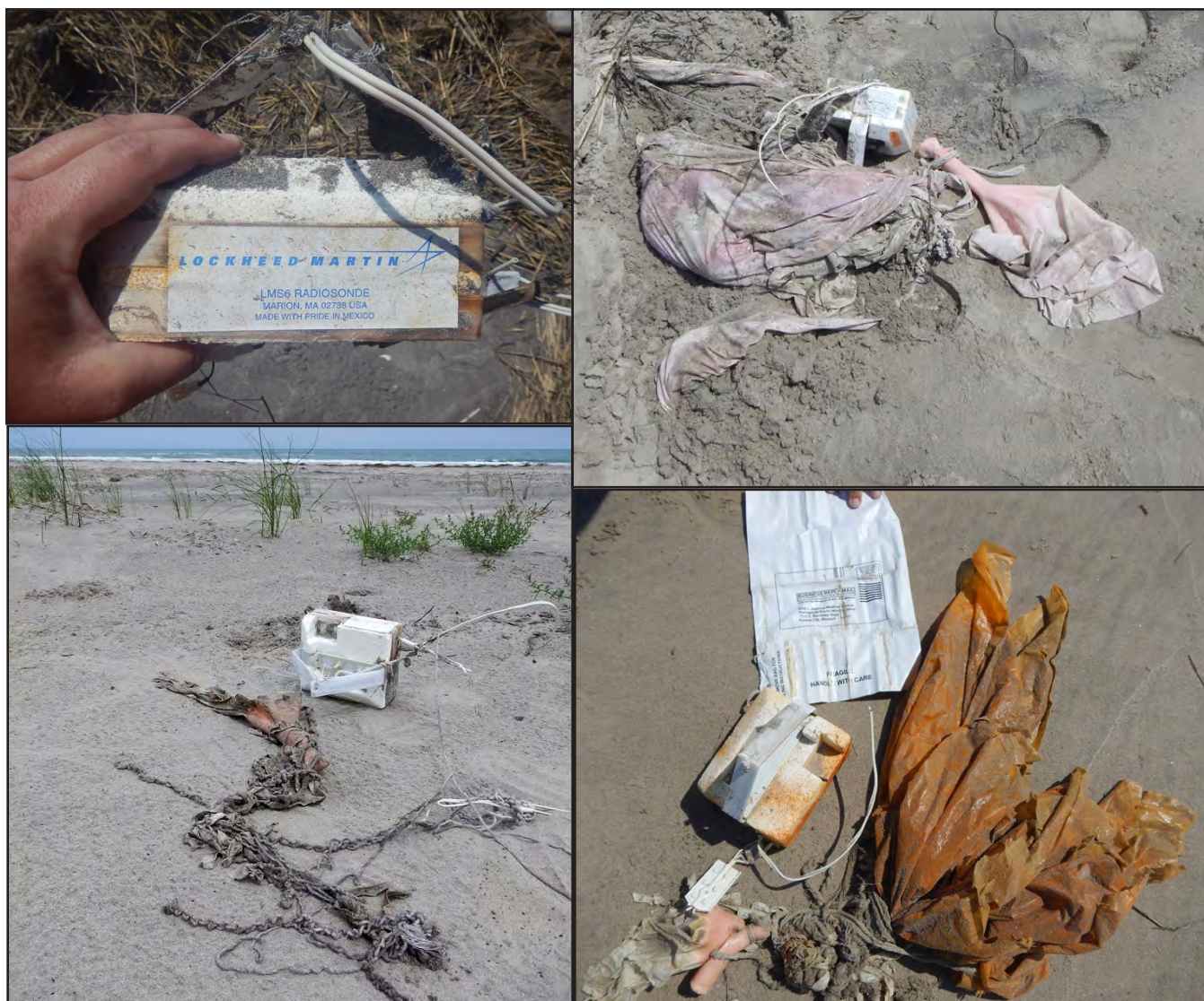
Weather balloon findings examples: (clockwise from top left) A Lockheed Martin radiosonde box; A radiosonde box attached to a large latex balloon with cotton string; A NOAA National Weather Service balloon including box, string, balloon, parachute and plastic return envelope; A radiosonde box with a latex balloon piece and many feet of cotton string.
