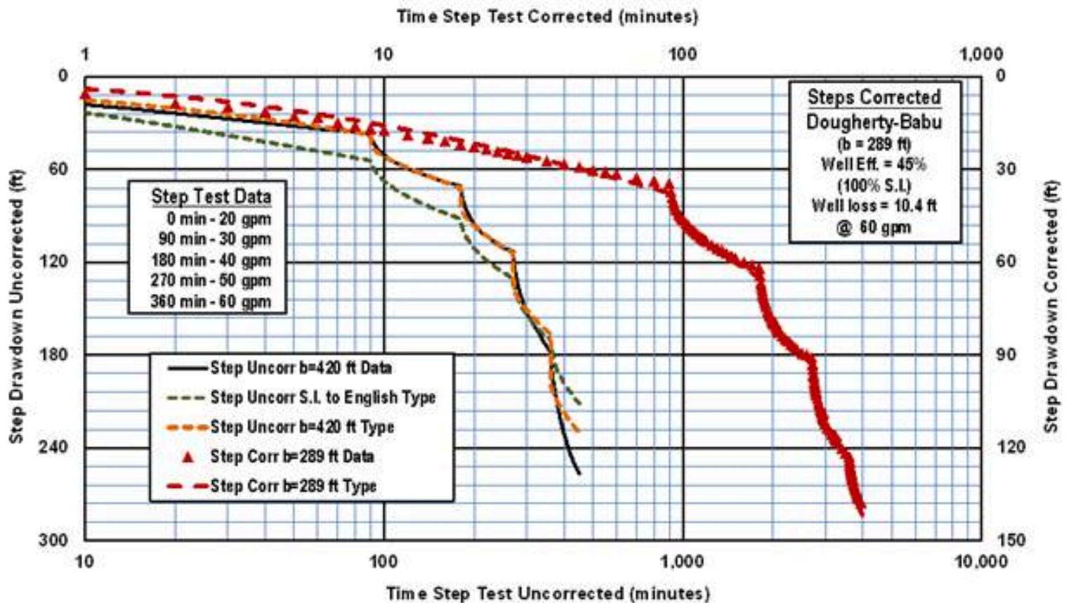
Figure A-8. Semi-log plot of drawdown from step-drawdown test of Poolesville well 7. Data is both uncorrected and corrected for aquifer thickness b of 289 ft. S.I. type curve converted to English units for uncorrected data.
