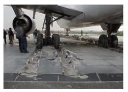
Engineered Materials Arrested System (EMAS)
